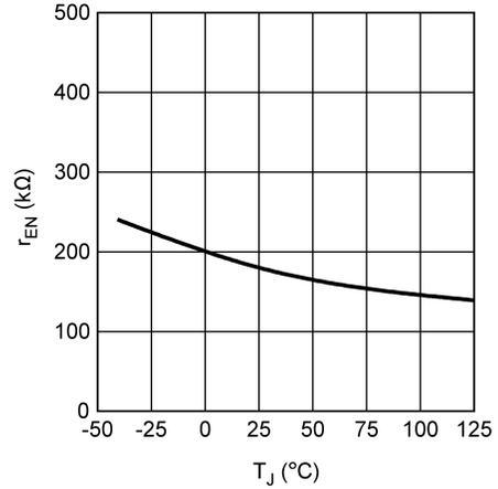
Figure 14. Enable Pullup Resistor ( $R_{EN}$ ) vs Temperature
