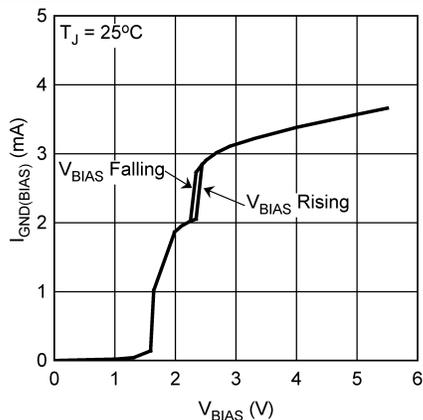
Figure 1.  $V_{BIAS}$  Ground Pin Current ( $I_{GND(BIAS)}$ ) vs  $V_{BIAS}$
