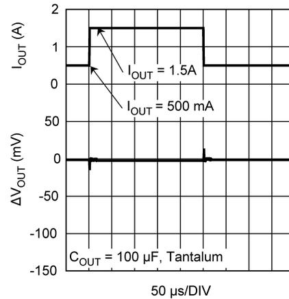
Figure 30. Load Transient Response
