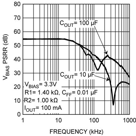
Figure 19.  $V_{BIAS}$  PSRR
