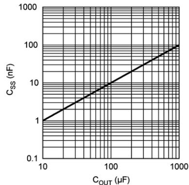
Figure 22. Typical C<sub>SS</sub> vs C<sub>OUT</sub> Values
