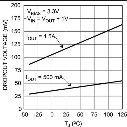
Figure 5. Dropout Voltage ( $V_{DO}$ ) vs Temperature
