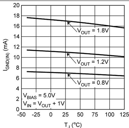
Figure 3.  $V_{IN}$  Ground Pin Current vs Temperature
