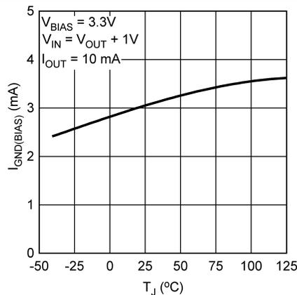
Figure 2.  $V_{BIAS}$  Ground Pin Current ( $I_{GND(BIAS)}$ ) vs Temperature
