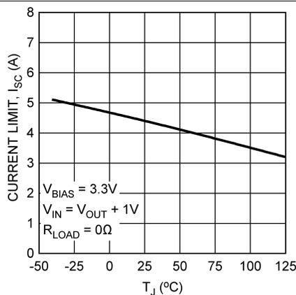
Figure 6. Output Current Limit ( $I_{SC}$ ) vs Temperature
