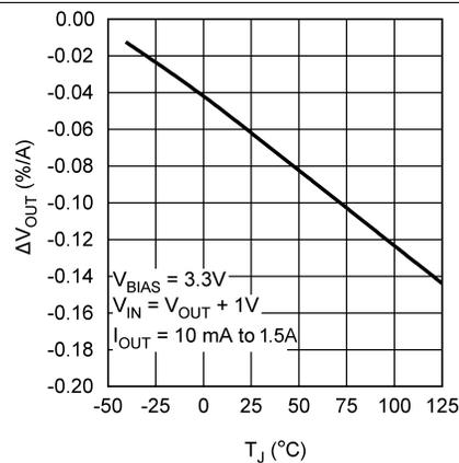
Figure 4. Load Regulation vs Temperature
