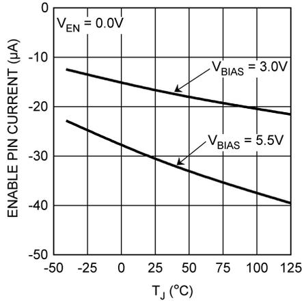
Figure 13. Enable Pulldown Current ( $I_{EN}$ ) vs Temperature
