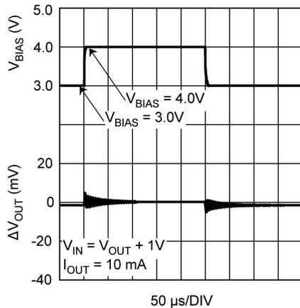
Figure 17.  $V_{BIAS}$  Line Transient Response
