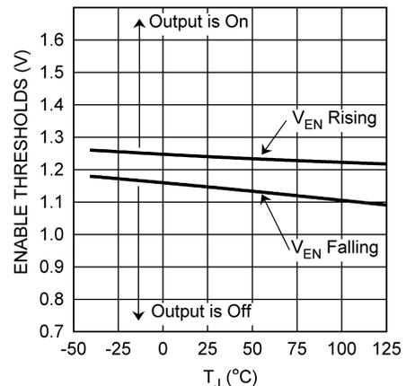
**Figure 12. Enable Thresholds ( $V_{EN}$ ) vs Temperature**
