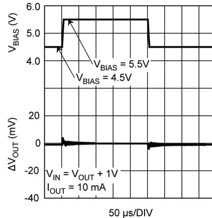
Figure 18.  $V_{BIAS}$  Line Transient Response
