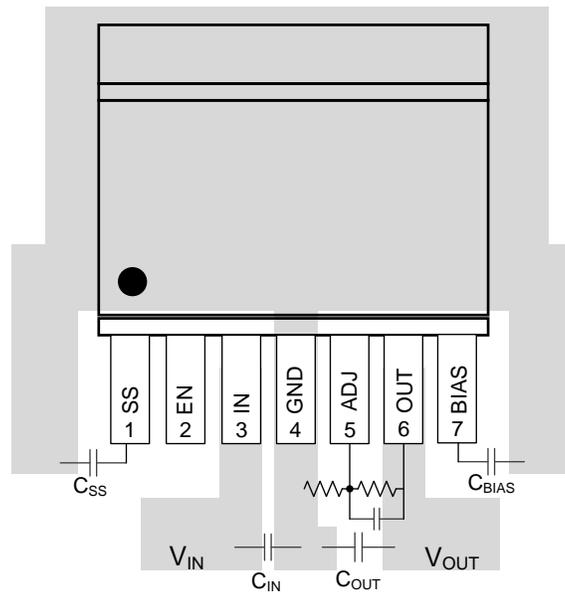
**Figure 31. LP38852 DDPAK/TO-263 and TO-220 Layout Example**
