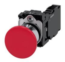
Mushroom pushbutton, 22 mm, round, metal, shiny, red, 40mm, latching, pull-to-unlatch mechanism, with holder, 1 NO+1 NC, screw terminal, with laser labeling, lower case
