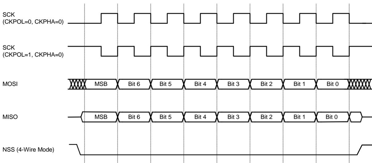
**Figure 18.6. Slave Mode Data/Clock Timing (CKPHA = 0)**
