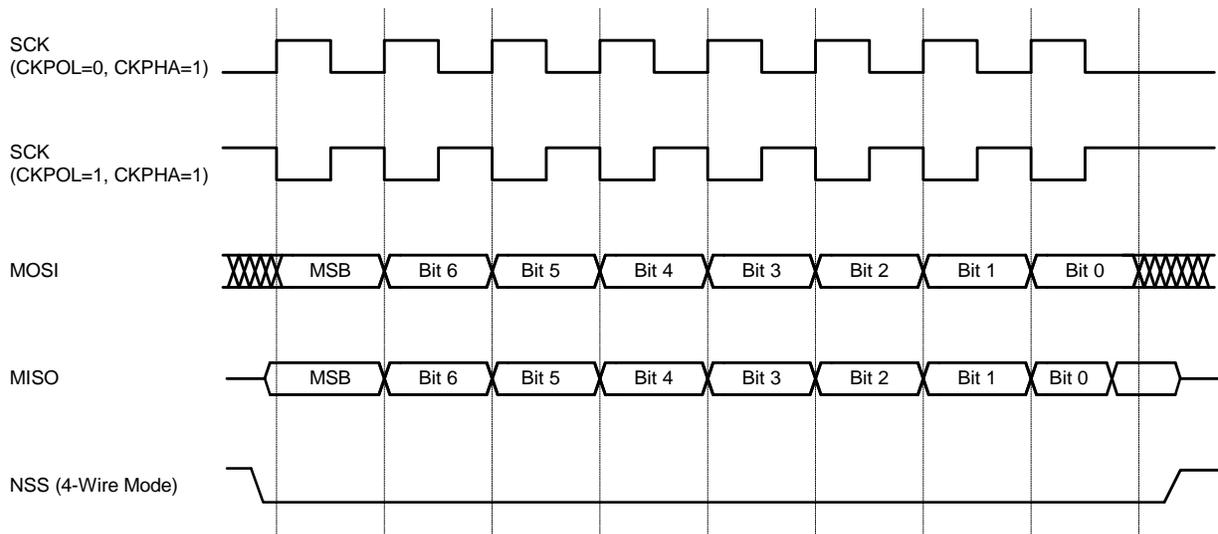
**Figure 18.7. Slave Mode Data/Clock Timing (CKPHA = 1)**
