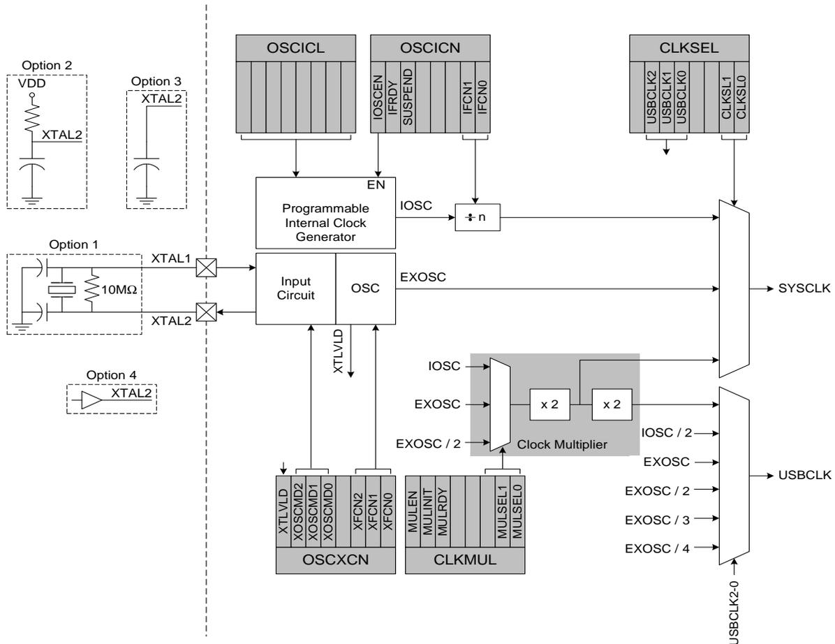
**Figure 13.1. Oscillator Diagram**
