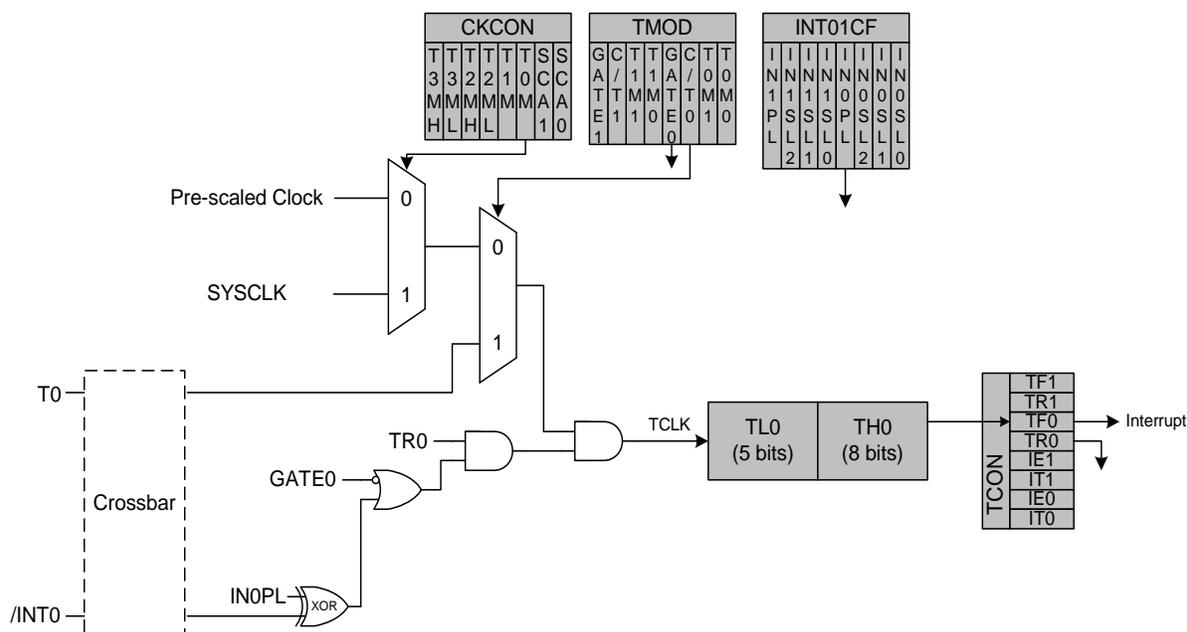
**Figure 19.1. T0 Mode 0 Block Diagram**
