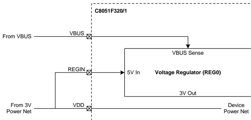
**Figure 8.4. REG0 Configuration: USB Self-Powered, Regulator Disabled**
