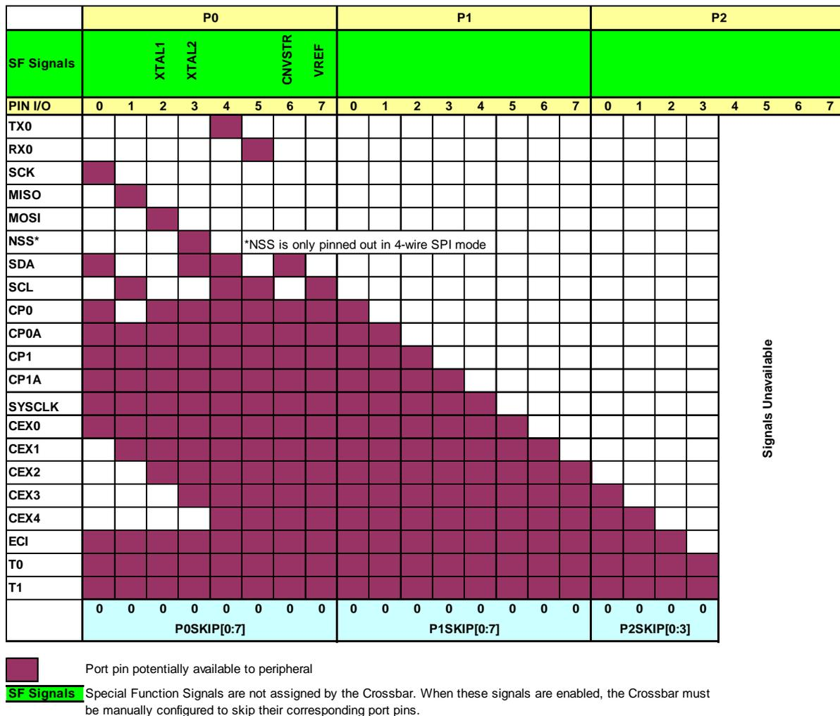
Figure 14.3. Crossbar Priority Decoder with No Pins Skipped
