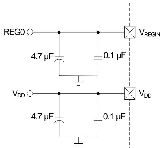
**Figure 8.1. External Capacitors for Voltage Regulator Input/Output**
