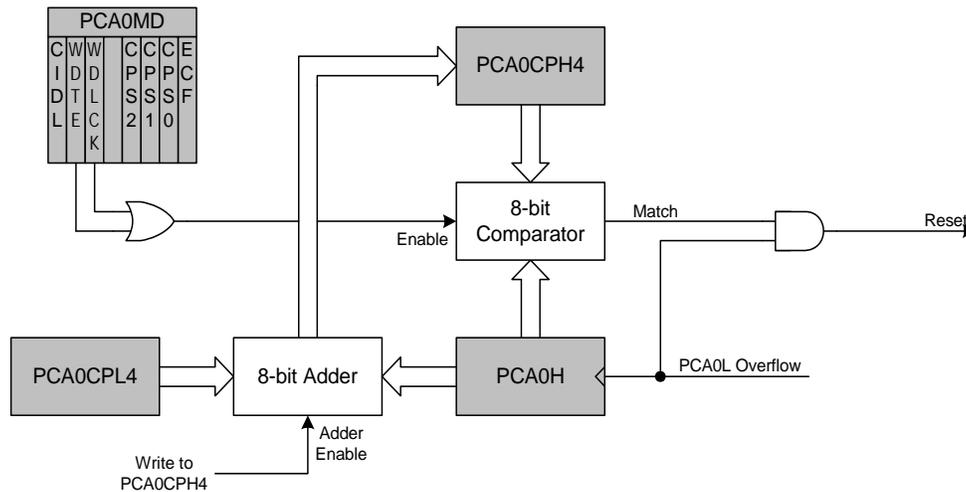
**Figure 20.10. PCA Module 4 with Watchdog Timer Enabled**
