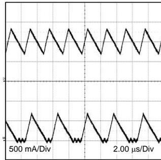
$V_{IN} = 12 \text{ V}, V_O = 3.3 \text{ V}, I_O = 3 \text{ A}/0.4 \text{ A } 2 \mu\text{s/div}$
