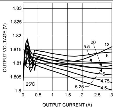
Figure 11. Line and Load Regulation at 25°C
