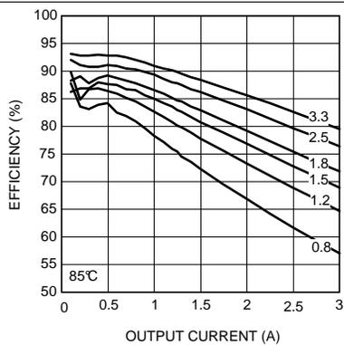
**Figure 5. Efficiency 6-V Input at 85°C**
