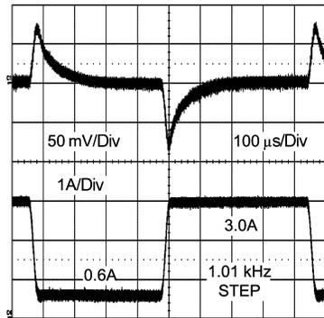
12  $V_{IN}$  3.3  $V_O$  0.6-A to 3-A Step
