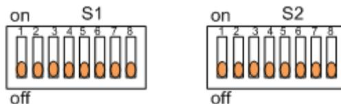
Figure 14: S1 and S2 configuration for external application control through USB
