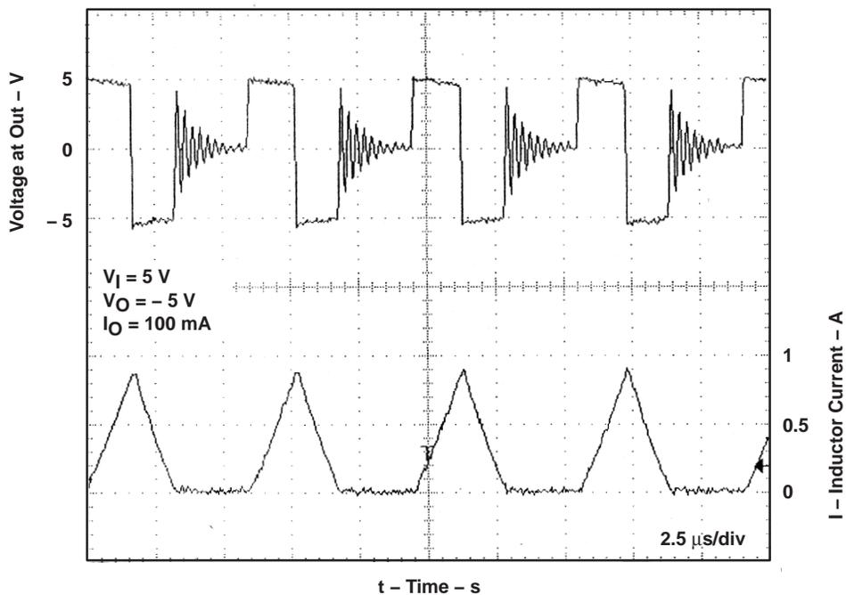
**Figure 2. Switching Waveforms**
