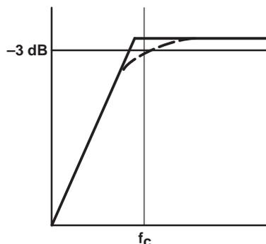
The value of  $C_1$  is important to consider as it directly affects the bass (low frequency) performance of the circuit. Consider the example where  $R_1$  is 10 k $\Omega$  and the specification calls for a flat bass response down to 40 Hz. Equation 8 is reconfigured as equation 10.
