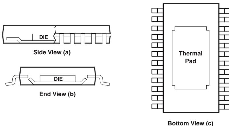
**Figure 58. Views of Thermally Enhanced PWP Package**
