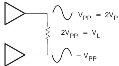
$$\text{Efficiency of a BTE Configuration} = \frac{P_L}{P_{\text{SUP}}} = \frac{V_{PP}^2}{2R_L} \times \frac{\pi R_L}{V_{DD} V_{PP}} = \frac{V_{PP} \pi}{2V_{DD}} = \frac{\pi \sqrt{2P_L R_L}}{2V_{DD}} \quad (4)$$
