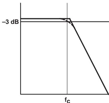
For example, if  $R_F$  is 100 k $\Omega$  and  $C_f$  is 5 pF then  $f_c$  is 318 kHz, which is well outside of the audio range.
