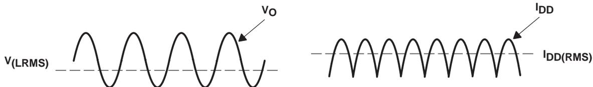
Figure 61. Voltage and Current Waveforms for BTL Amplifiers
