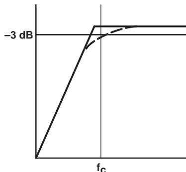
The main disadvantage, from a performance standpoint, is the load impedances are typically small, which drives the low-frequency corner higher degrading the bass response. Large values of  $C_C$  are required to pass low frequencies into the load. Consider the example where a  $C_C$  of 330  $\mu\text{F}$  is chosen and loads vary from 4  $\Omega$ , 8  $\Omega$ , 32  $\Omega$ , to 47 k $\Omega$ . Table 2 summarizes the frequency response characteristics of each configuration.
