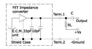
RL =  $2.2 \text{ k}\Omega$ C =  $1 \mu\text{F}$
