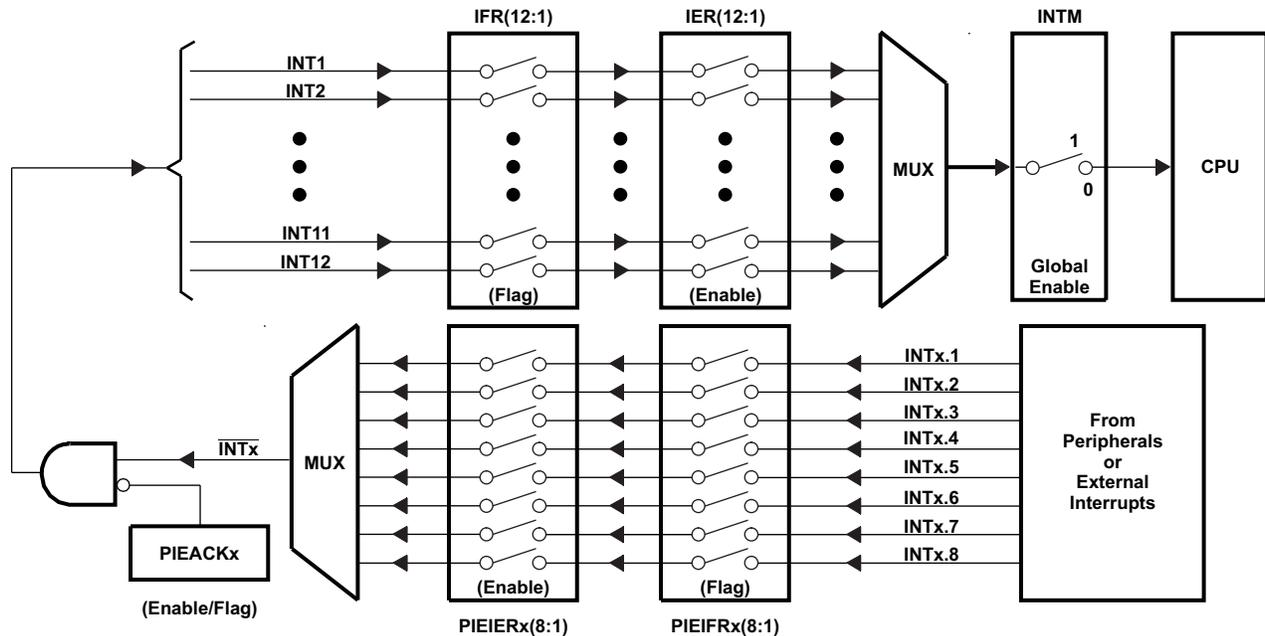
Figure 6-15. Multiplexing of Interrupts Using the PIE Block
