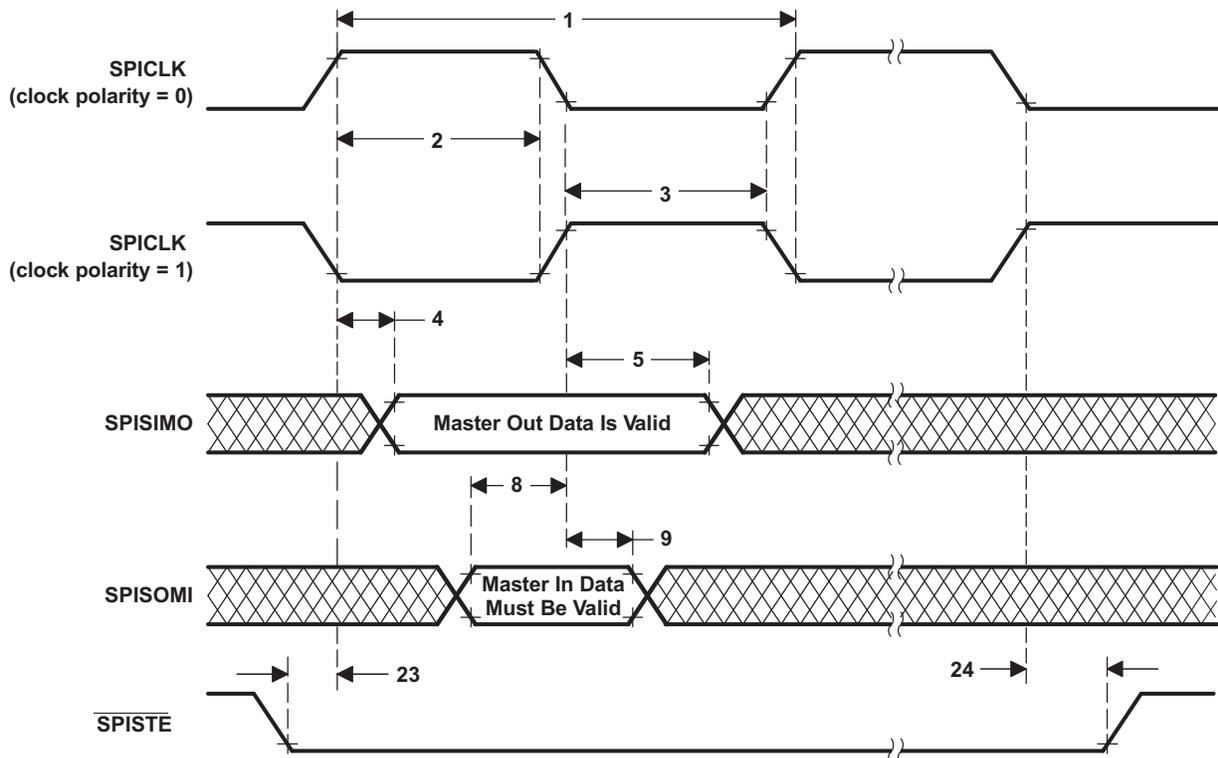
**Figure 5-15. SPI Master Mode External Timing (Clock Phase = 0)**
