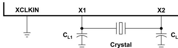
Figure 6-20. Using the Internal Oscillator
