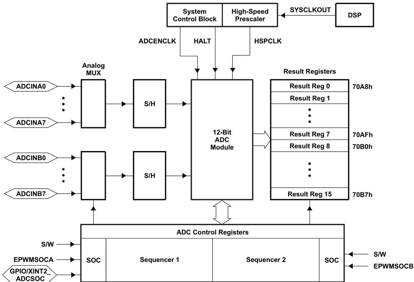
Figure 6-5. Block Diagram of the ADC Module
