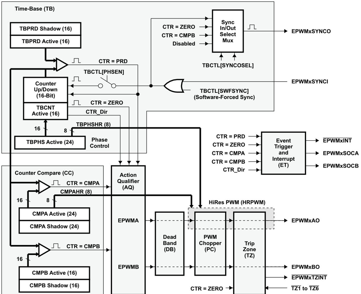
Figure 6-4. ePWM Sub-Modules Showing Critical Internal Signal Interconnections
