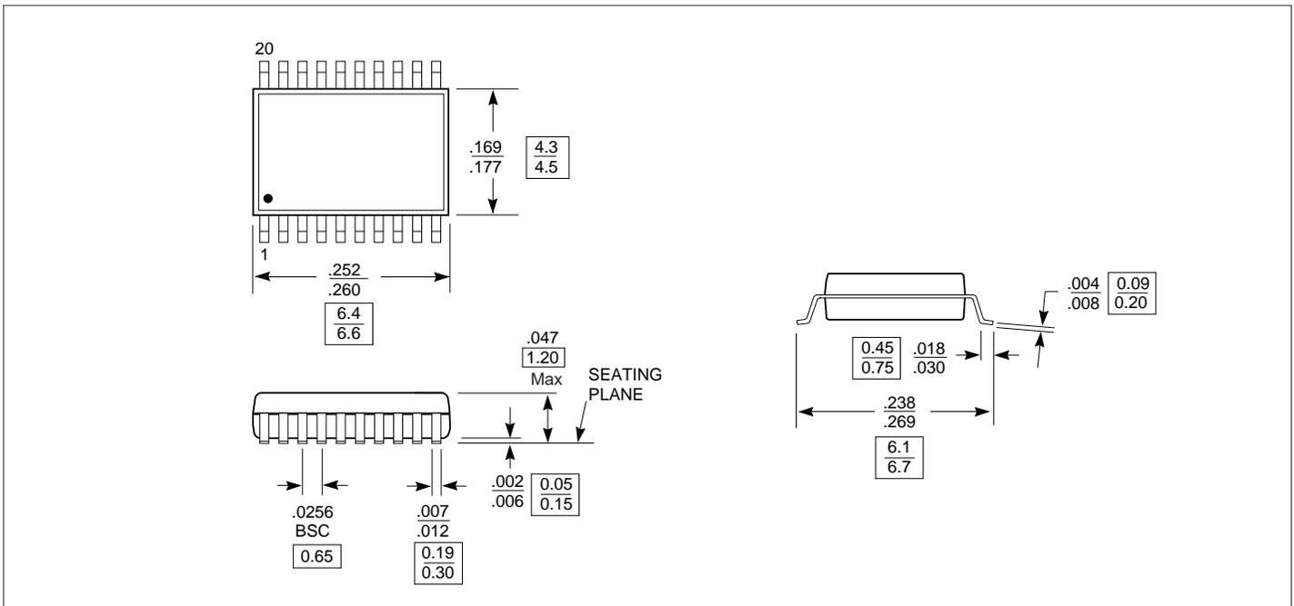
**Packaging Mechanical: 20-Pin SOIC(S)**
