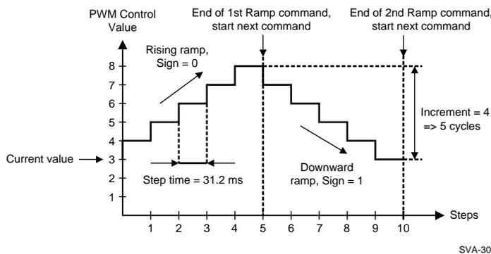
**Figure 16. Example of 2 Sequential Ramp Commands**
