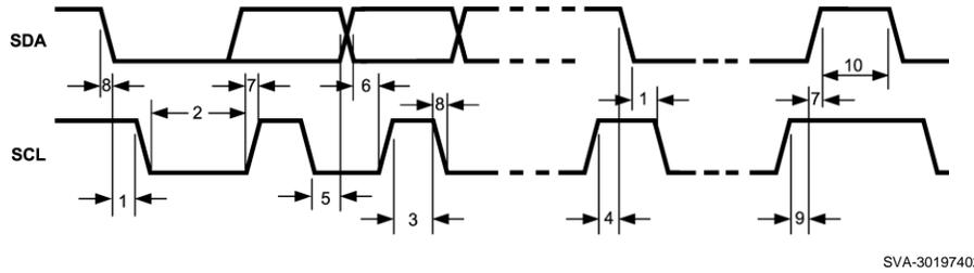
**Figure 2. I<sup>2</sup>C Timing Parameters**
