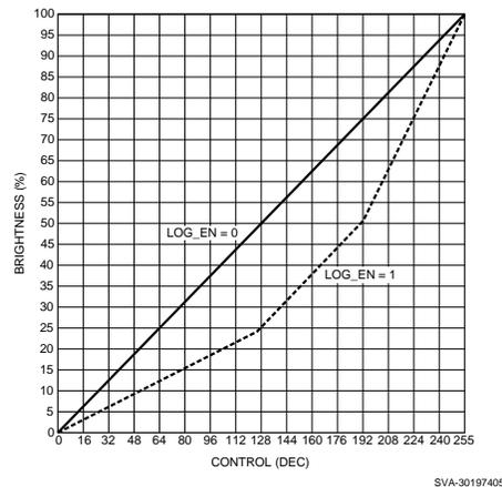
Figure 15. Logarithmic and Linear PWM Adjustment Curves
