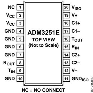
Figure 2. Pin Configuration
