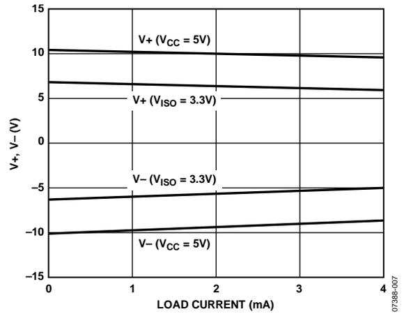
Figure 7. Charge Pump  $V_+$ ,  $V_-$  vs. Load Current
