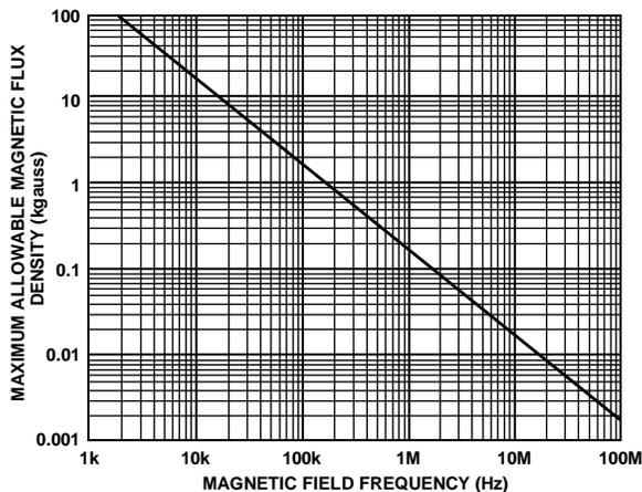
Figure 22. Maximum Allowable External Magnetic Flux Density
