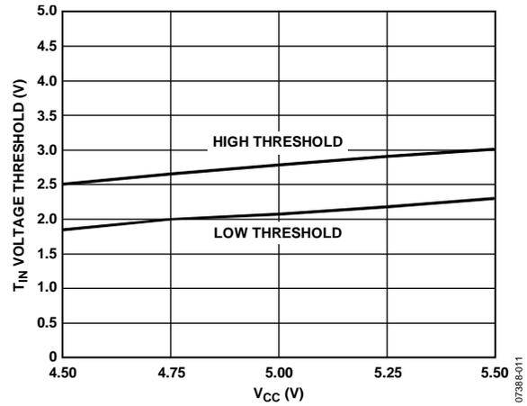
Figure 12. T<sub>IN</sub> Voltage Threshold vs. V<sub>CC</sub>
