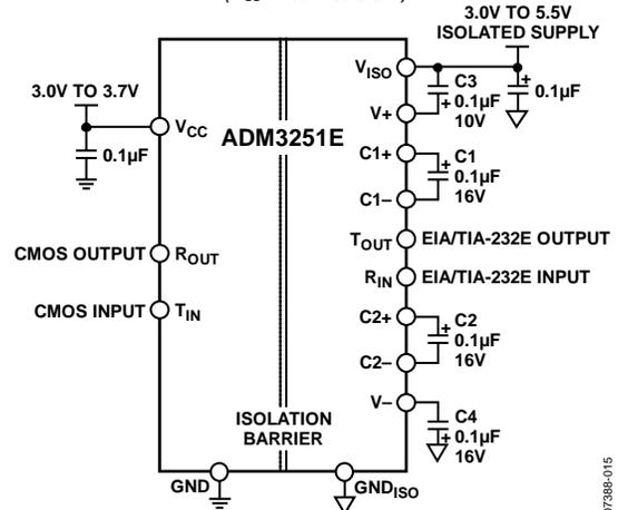
Figure 15. Typical Operating Circuit with the DC-to-DC Converter Disabled (V<sub>CC</sub> = 3.0 V to 3.7 V)
