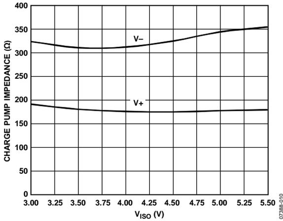
Figure 9. Charge Pump Impedance vs. V<sub>ISO</sub>
