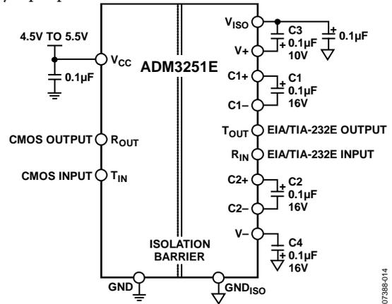
Figure 14. Typical Operating Circuit with the DC-to-DC Converter Enabled (V<sub>CC</sub> = 4.5 V to 5.5 V)
