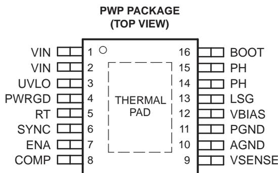
NOTE: If there is not a pin 1 indicator, turn device to enable reading the symbol from left to right. Pin 1 is at the lower left corner of the device.
