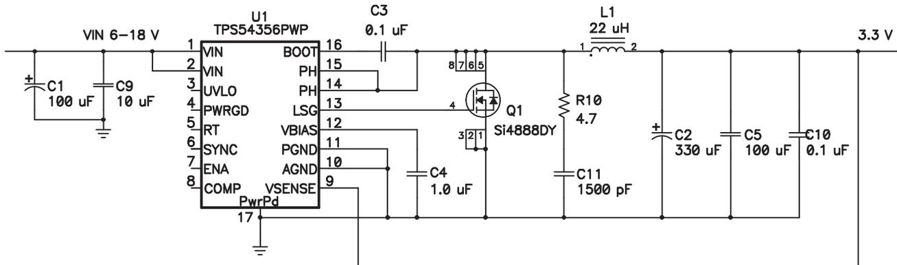
Figure 25. Application Circuit, 12 V to 3.3 V
