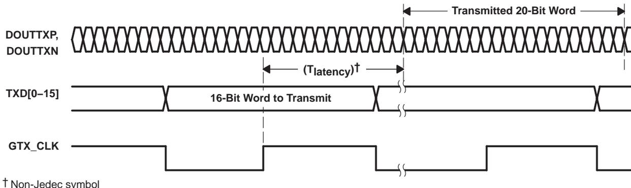
Figure 3. Transmitter Latency
