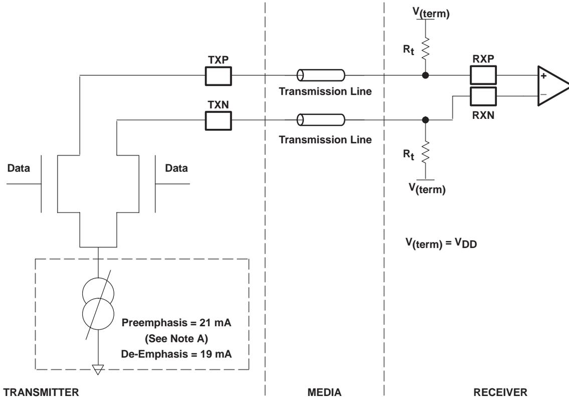
NOTE A: This assumes  $R_{REF} = 200 \Omega$  and termination resistance =  $50 \Omega$ . See Figure 14 and section *choosing RREF resistor values* for more information.
