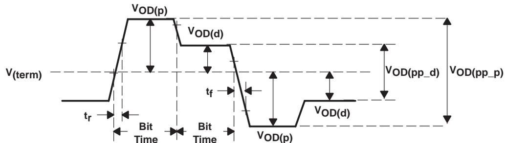
Figure 12. Differential and Common-Mode Output Voltage Definitions
