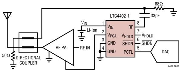
Dual Band Cellular Telephone Transmitter
