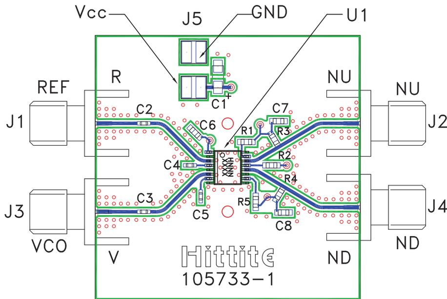
The circuit board used in the final application should use RF circuit design techniques. Signal lines should have 50 ohm impedance while the package ground leads and backside ground slug should be connected directly to the ground plane similar to that shown. A sufficient number of via holes should be used to connect the top and bottom ground planes. The evaluation circuit board shown is available from Hittite upon request.
