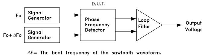
**Typical PLL Application Circuit using HMC439QS16G**
