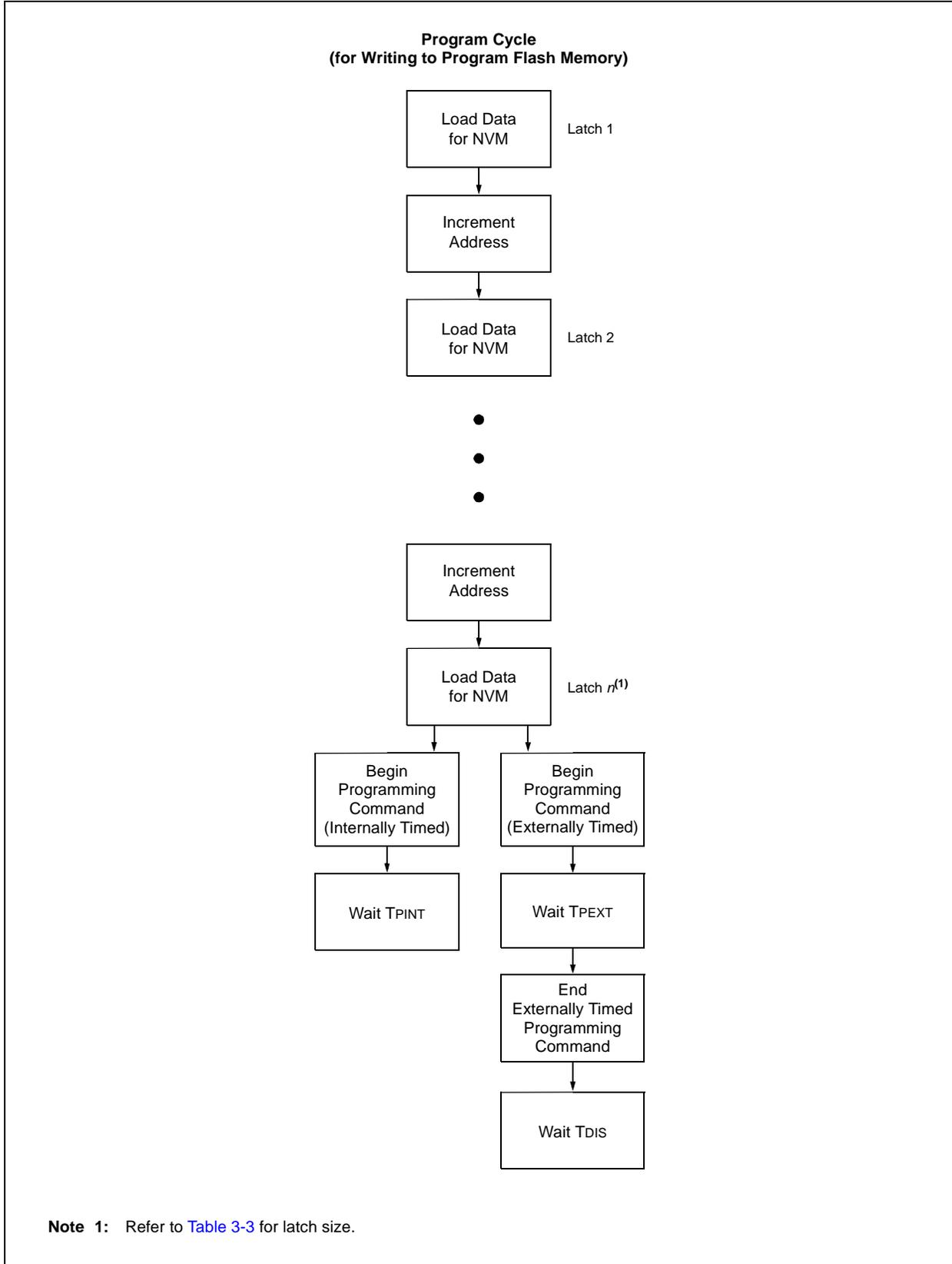
**FIGURE 3-21: USER ID AND CONFIGURATION MEMORY PROGRAM FLOWCHART**
