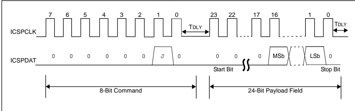
**FIGURE 3-7: LOAD DATA FOR NVM (DATA EEPROM)**
