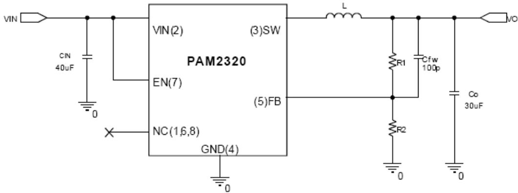
$$V_O = 0.6 \times \left( 1 + \frac{R_1}{R_2} \right)$$
