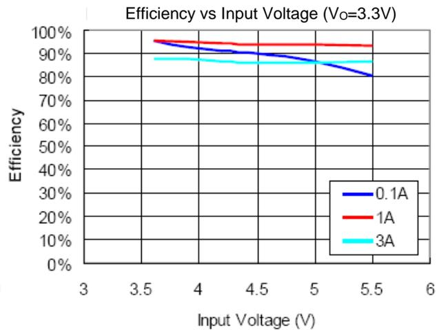
**Typical Performance Characteristics** (continued) (@ $T_A = +25^\circ\text{C}$ ,  $C_{IN} = 33\mu\text{F}$ ,  $C_O = 22\mu\text{F}$ , unless otherwise specified.)
