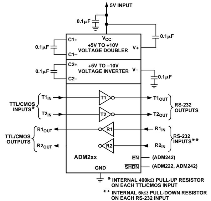
functions are disabled. The ADM222 is available in 18-lead DIP and in a wide surface-mount (SOIC) package.
