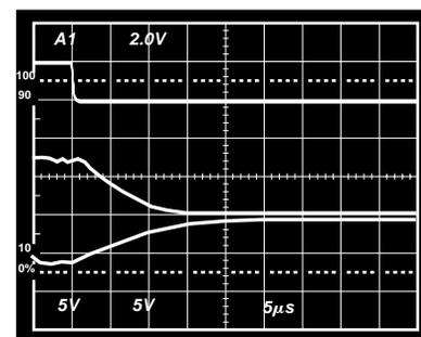
Figure 13. Transmitter Output Disable Timing
