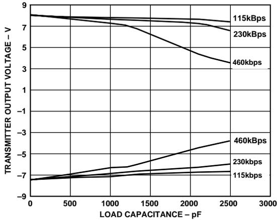
TPC 2. Transmitter Baud Rate vs. Load Capacitance
