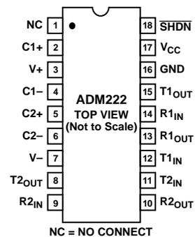
Figure 8. ADM222 DIP and SOIC Pin Configurations
