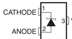
\*Pin 3 is attached to Substrate and must be connected to ANODE or left open.
