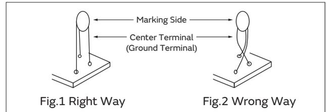
3. Take care not to apply any mechanical stress to product body at the lead terminal bending process for product angle adjustment after insertion.
