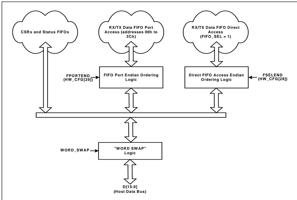
Data path operations for the various supported endianness and word swap configurations are illustrated in [Figure 3-9](#). [Table 3-8, "Endian Ordering Logic Operation"](#) illustrates the byte ordering applied by the endian logic for each type of host access. This figure and table assume an internal byte ordering of 3-2-1-0, where '3' is the most significant byte (data[31:24]) and '0' is the least significant byte (data[7:0]).
