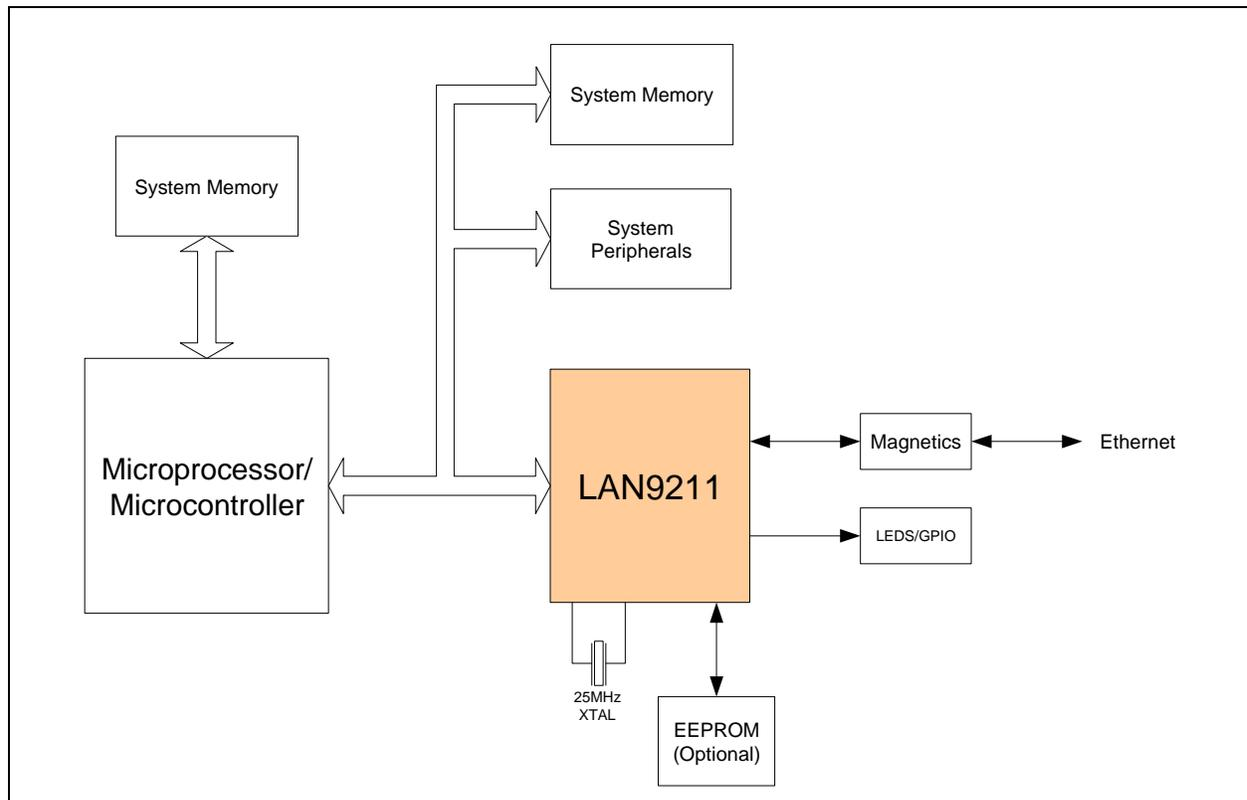
The Microchip LAN9211 integrated 10/100 MAC/PHY controller is a peripheral chip that performs the function of translating parallel data from a host controller into Ethernet packets. The LAN9211 Ethernet MAC/PHY controller is designed and optimized to function in an embedded environment. All communication is performed with programmed I/O transactions using the simple SRAM-like host interface bus.
