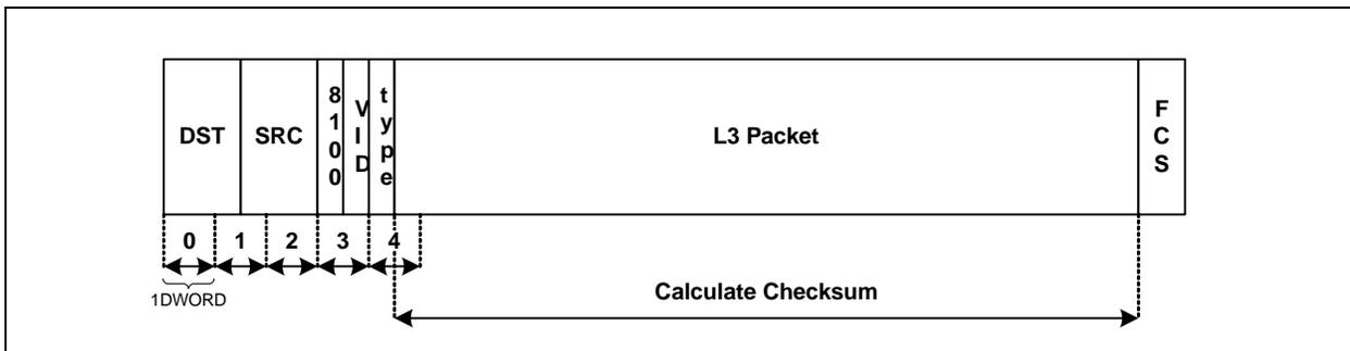
**FIGURE 3-5: ETHERNET FRAME WITH LENGTH FIELD AND SNAP HEADER**
