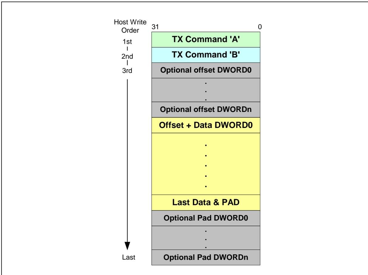
Figure 3-20, "TX Buffer Format", shows the TX Buffer as it is written into the LAN9211. It should be noted that not all of the data shown in this diagram is actually stored in the TX data FIFO. This must be taken into account when calculating the actual TX data FIFO usage. Please refer to [Section 3.12.5, "Calculating Actual TX Data FIFO Usage," on page 46](#) for a detailed explanation on calculating the actual TX data FIFO usage.
