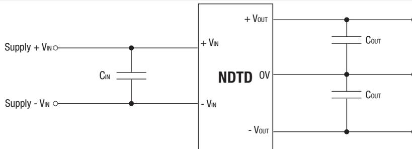
**Reflected Ripple Current Measurement**
