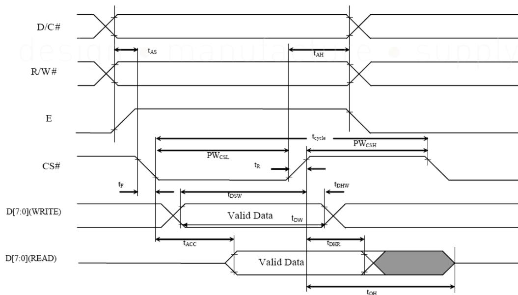
80XX-Series MPU Parallel Interface Timing Characteristics:
