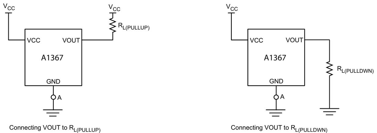
Figure 11: Connections for Detecting Broken Ground Wire
