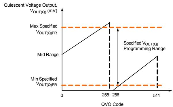
Figure 8: Device  $V_{OUT(Q)}$  versus QVO Programmed Value
