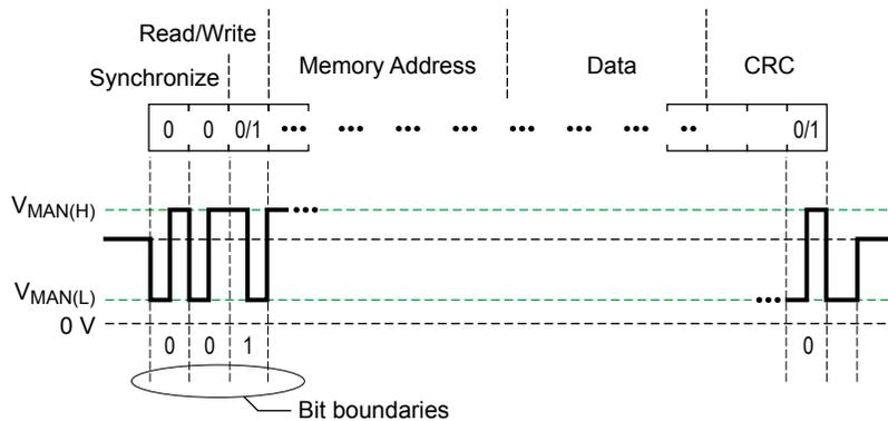
Figure 13: General Format for Serial Interface Commands
