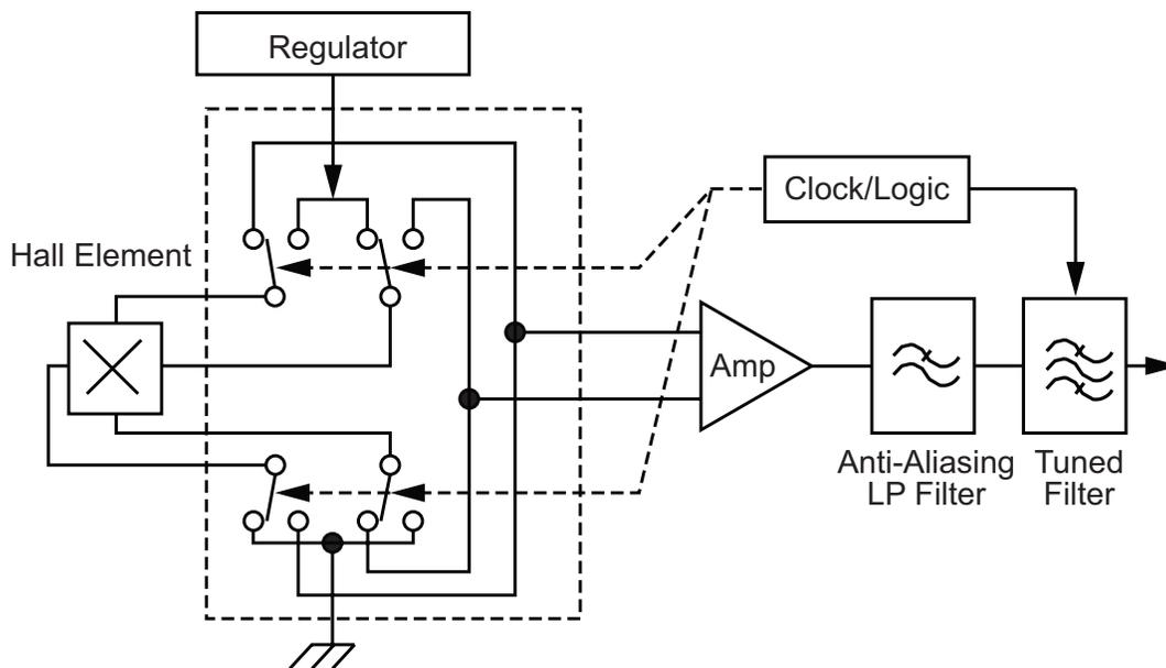
Figure 12: Concept of Chopper Stabilization
