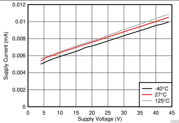
Figure 6. Standby Recessive  $I_{SUP}$  vs  $V_{SUP}$  and Temperature
