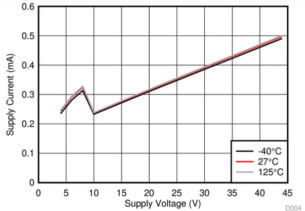
Figure 4. Recessive  $I_{SUP}$  vs  $V_{SUP}$  and Temperature
