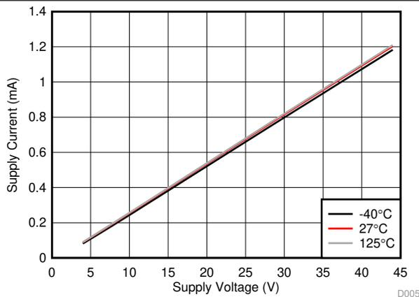
Figure 5. Standby Dominant  $I_{SUP}$  vs  $V_{SUP}$  and Temperature
