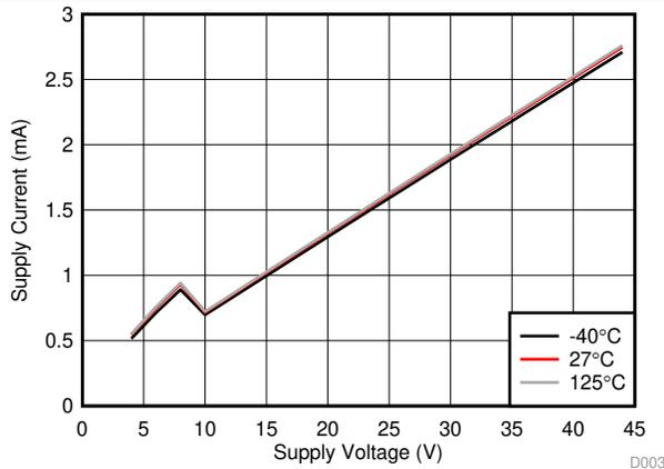
Figure 3. Dominant  $I_{SUP}$  vs  $V_{SUP}$  and Temperature
