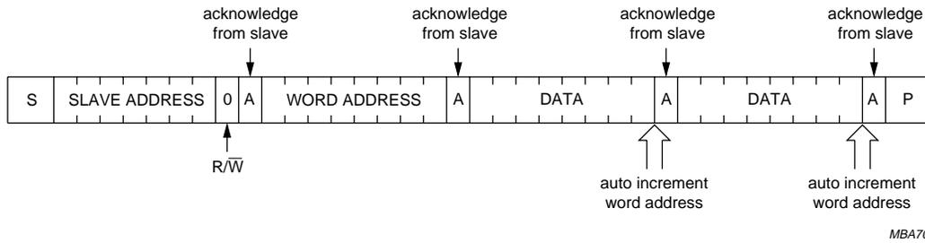
Fig 5. Auto-increment memory word address; two byte write.
