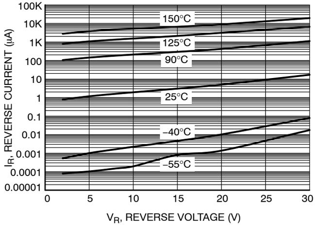
Figure 6. Leakage Current
