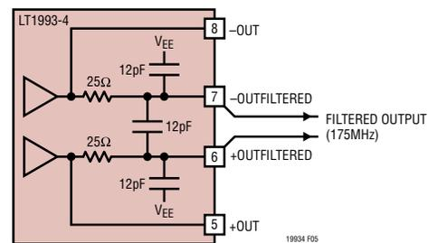
Figure 5. LT1993-4 Internal Filter Topology -3dB BW ≈175MHz
