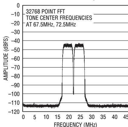
4-Tone WCDMA Waveform LT1993-4 Driving LTC2255 14-Bit ADC at 92.16Mps
