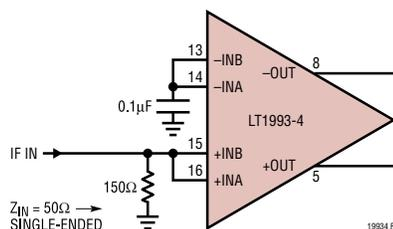
Figure 1. Input Termination for Single-Ended 50 $\Omega$  Input Impedance
