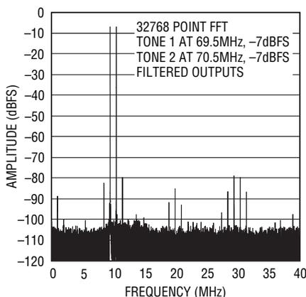
2-Tone WCDMA Waveform LT1993-4 Driving LTC2255 14-Bit ADC at 92.16Mps
