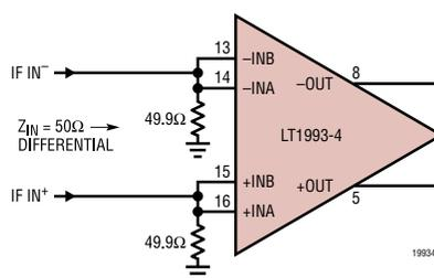
Figure 2. Input Termination for Differential 50 $\Omega$  Input Impedance
