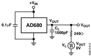
Figure 12. Capacitive Load Transient Response Test Circuit
