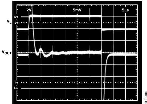
Figure 13. Output Response with Capacitive Load
