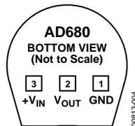
Figure 4. Connection Diagram
