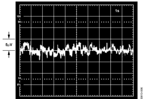
Figure 6. 0.1 Hz to 10 Hz Noise
