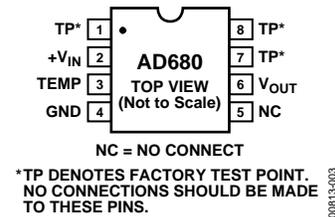
Figure 1. 8-Lead PDIP and 8-Lead SOIC Pin Configuration
