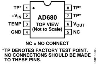
Figure 3. 8-Lead PDIP and 8-Lead SOIC Pin Configuration
