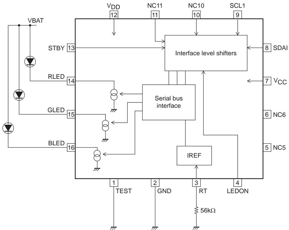
Note 1 : The TEST pin must be tied to ground.
