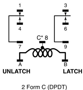
\* C denoted common connection. On 3-pole relays the common connection is a wire lead coming off of the coil. It is not terminated to the relay header. Consult your Omron representative for single coil or isolated double coil models.
