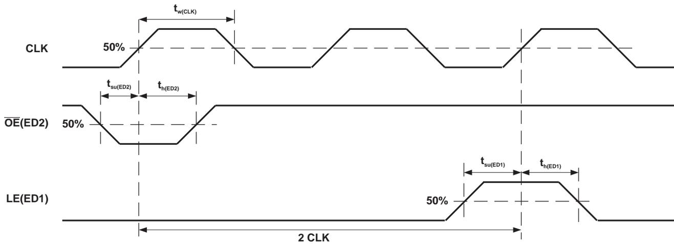
Figure 8. Switching to Special Mode Timing Waveforms
