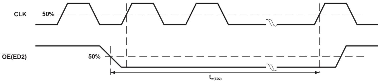
Figure 9. Reading Error Status Code Timing Waveforms
