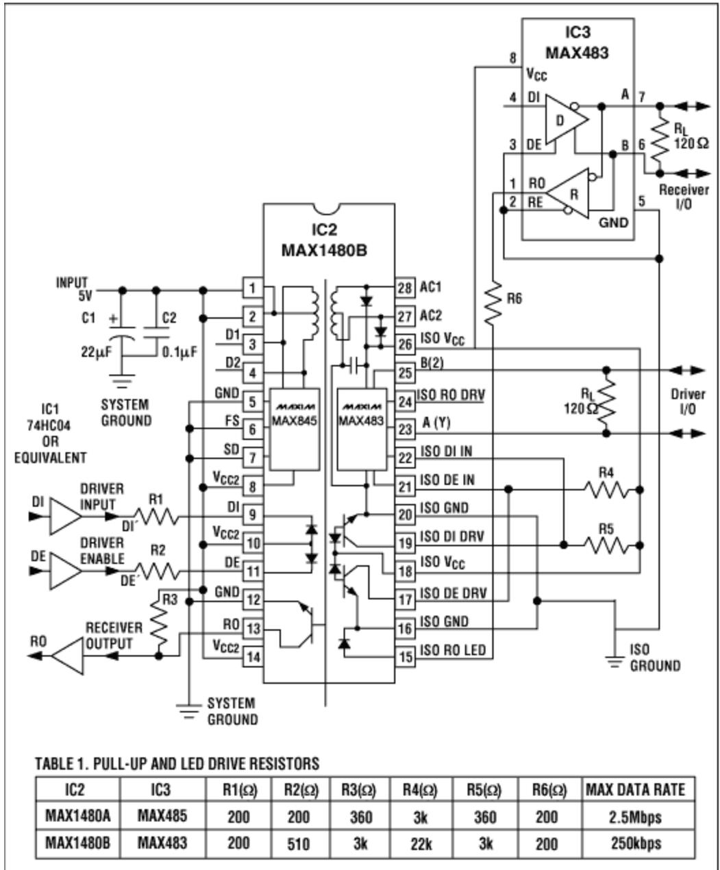
TABLE 1. PULL-UP AND LED DRIVE RESISTORS
