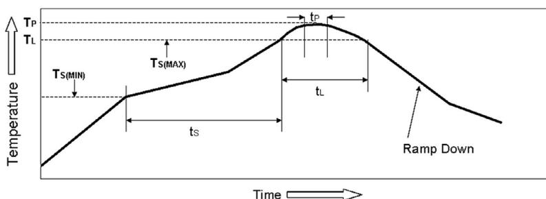
The Pb Free Process-Package Peak Reflow Temperature is 260°C.
