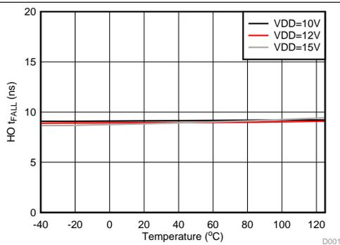
**Figure 12. HO Fall Time with 1000-pF Load vs Temperature**
