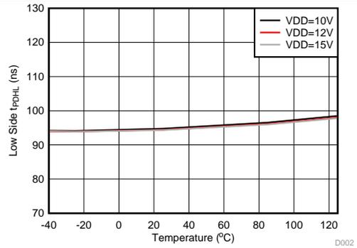
Figure 3. Low-Side, Turn-Off Propagation Delay vs Temperature
