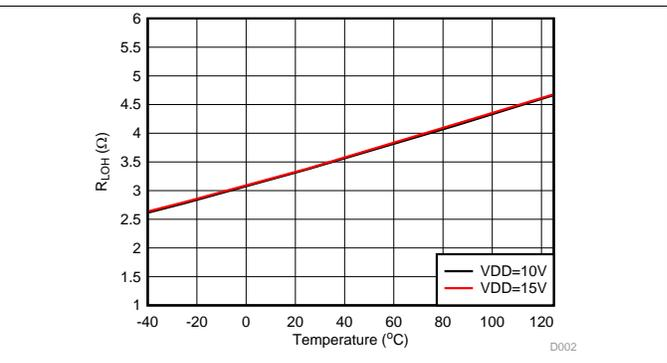
Figure 21. LO Output Pull-Up Resistance vs Temperature
