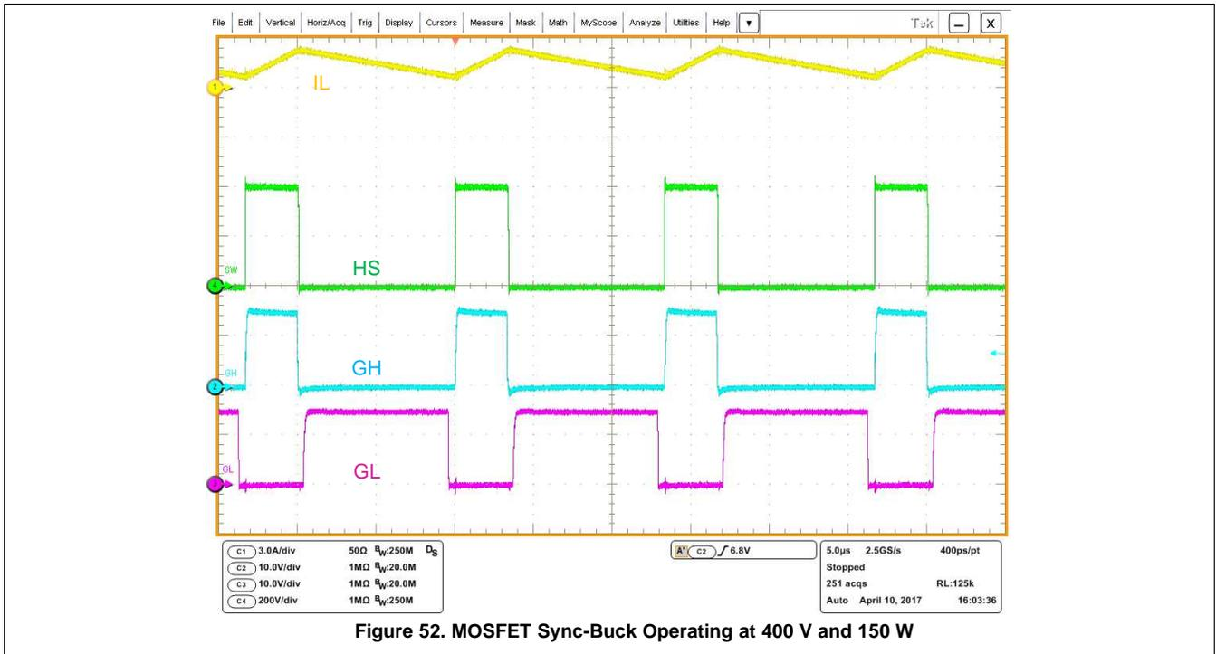
Figure 52. MOSFET Sync-Buck Operating at 400 V and 150 W
