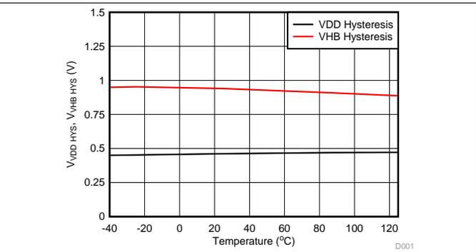
**Figure 15. VDD and VHB-VHS UVLO Hysteresis vs Temperature**
