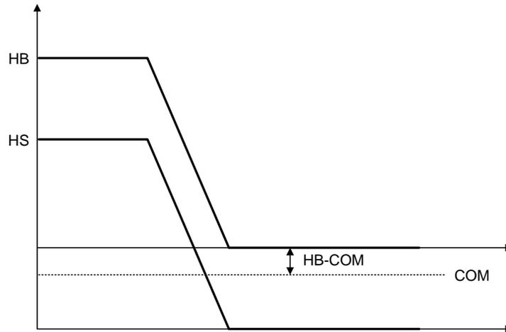
**Figure 41. Level Shifter Supply Voltage with Negative HS**
