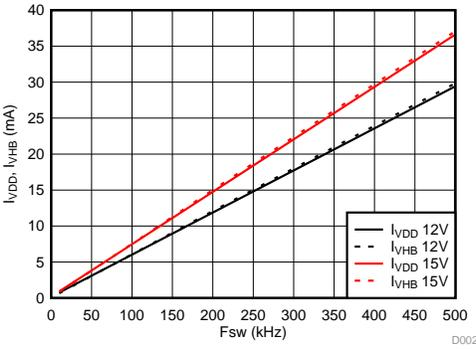
Figure 28. VDD and HB Operating Current with 4700-pF Load vs Switching Frequency
