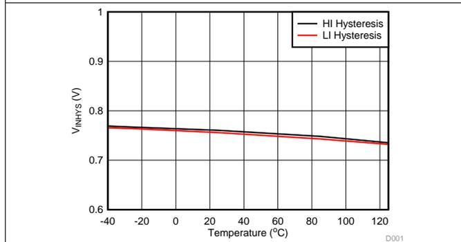
**Figure 18. HI/LI Pin Hysteresis vs Temperature**
