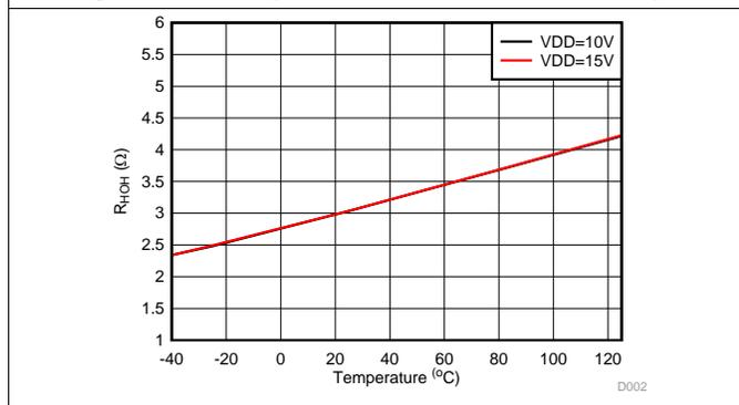
Figure 22. HO Output Pull-Up Resistance vs Temperature
