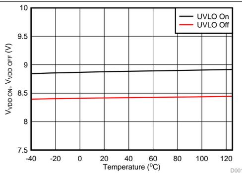
**Figure 13. VDD UVLO Thresholds vs Temperature**
