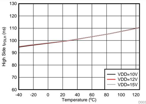
Figure 4. High-Side, Turn-On Propagation Delay vs Temperature
