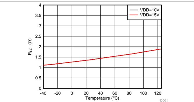
**Figure 19. LO Output Pull-Down Resistance vs Temperature**
