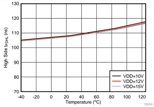
Figure 5. High-Side, Turn-Off Propagation Delay vs Temperature
