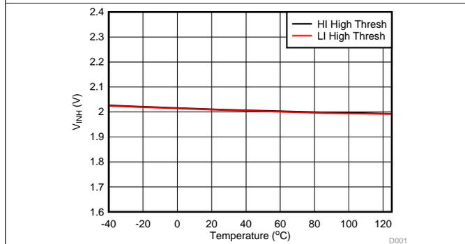
**Figure 16. HI/LI Pin High Threshold vs Temperature**
