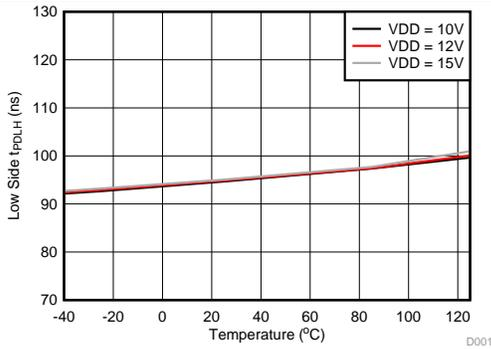
Figure 2. Low-Side, Turn-On Propagation Delay vs Temperature
