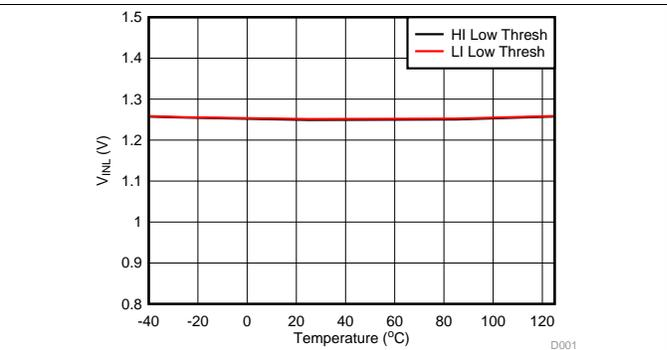
**Figure 17. HI/LI Pin Low Threshold vs Temperature**
