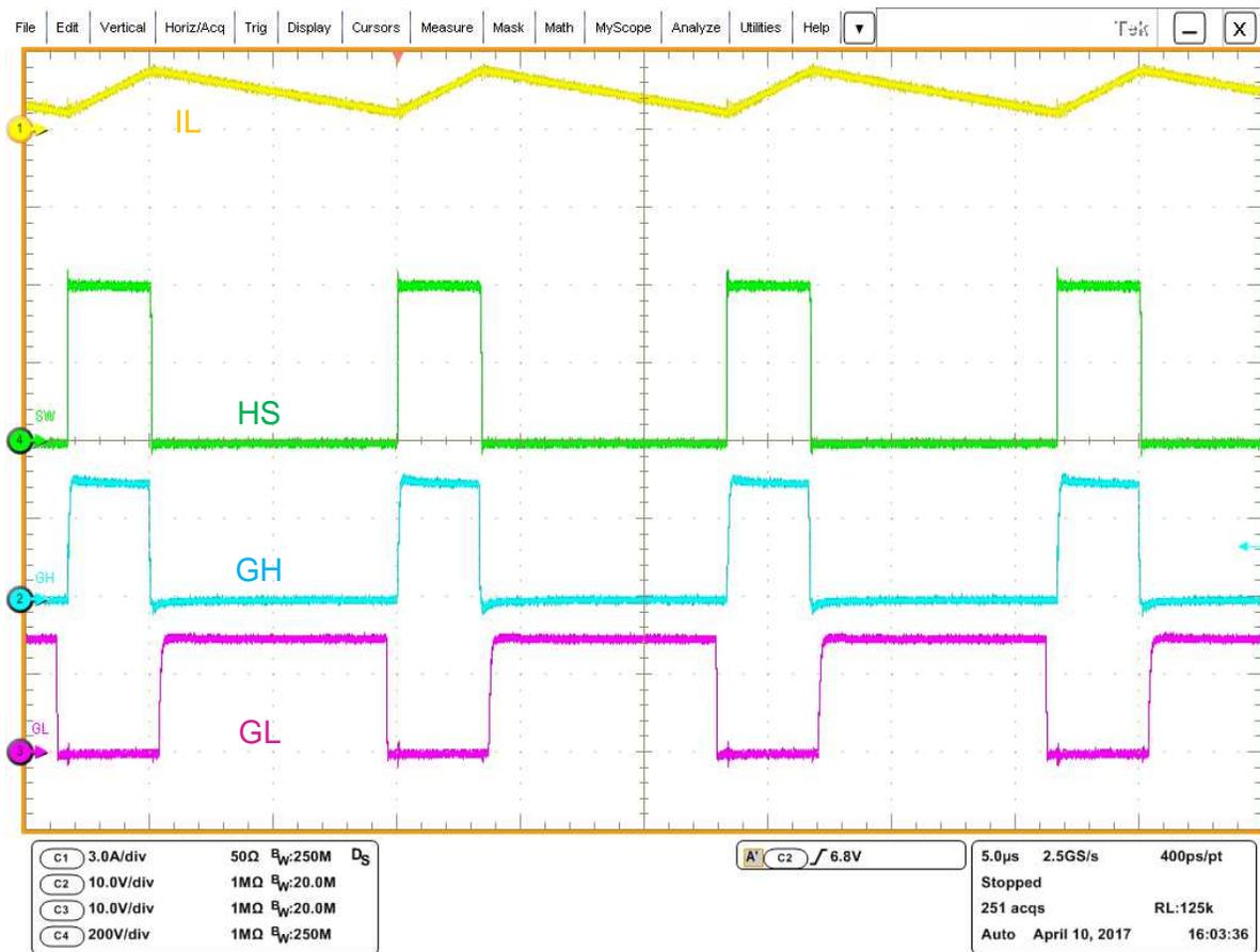
**Figure 47. IGBT Sync-Buck Operating at 400 V and 150 W**
