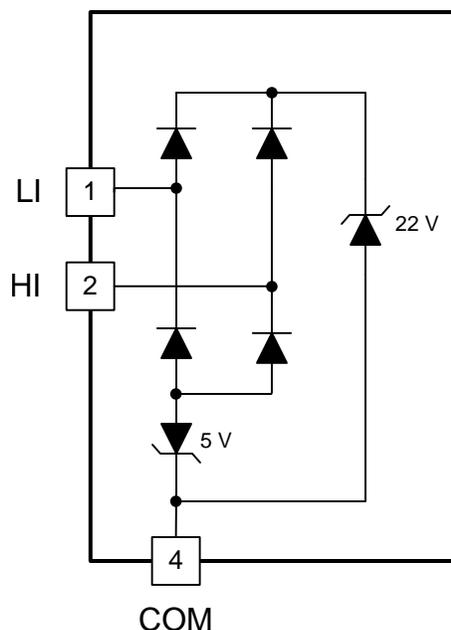
**Figure 31. Diode Structure of Input Stage**
