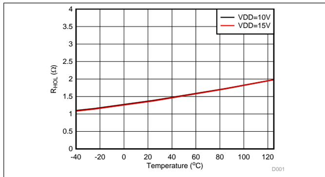
Figure 20. HO Output Pull-Down Resistance vs Temperature
