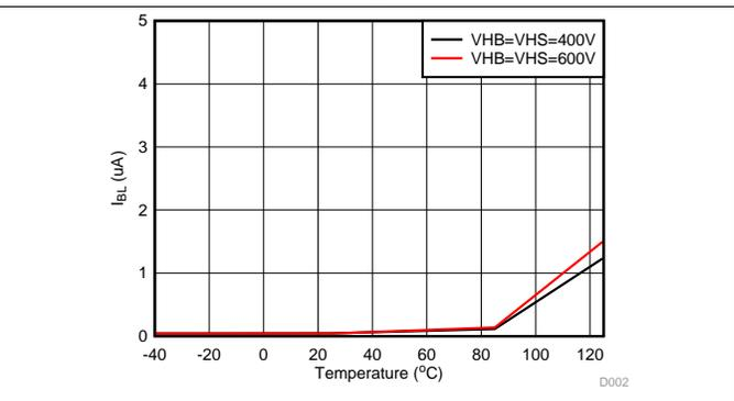
Figure 25. HB to COM Bootstrap Supply Leakage Current vs Temperature
