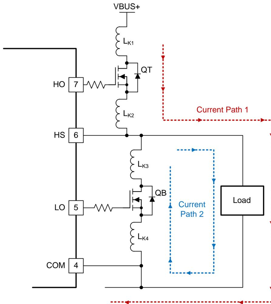
Figure 40. HS Negative Voltage In Half-Bridge Configuration
