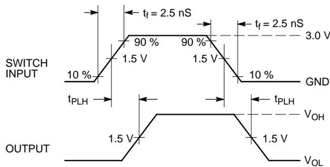
**Figure 5. Propagation Delays**
