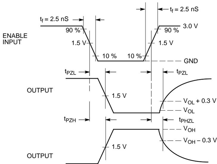
**Figure 6. Enable/Disable Delays**
