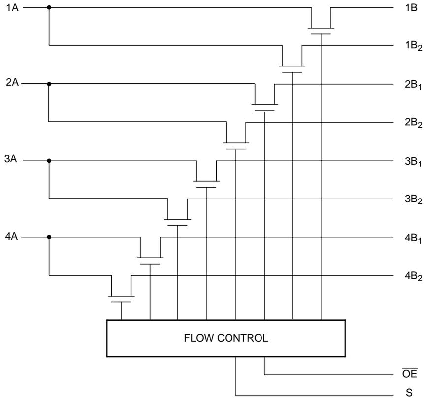
Figure 3. Logic Diagram
