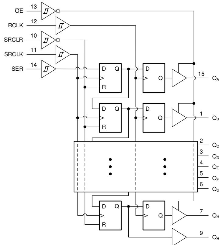
Figure 8-1. Logic Diagram (Positive Logic) for the SN74HCS595-Q1
