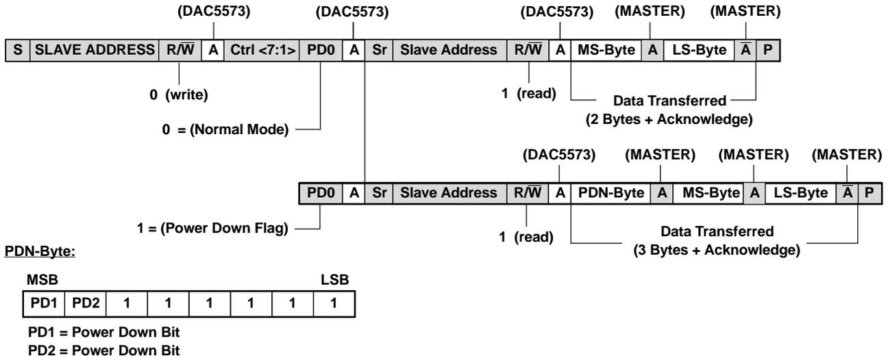
Figure 35. Standard and Fast Mode: Slave Transmitter
