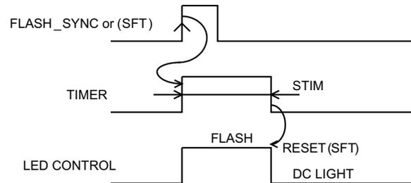
**Figure 51. Edge Sensitive Timer (Single Trigger Event)**
