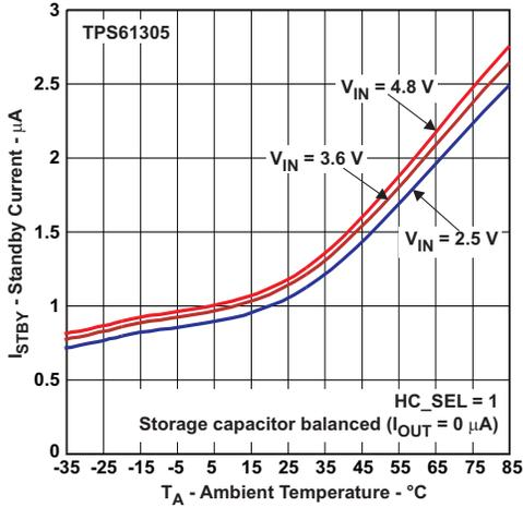
Figure 26. Standby Current vs Ambient Temperature (HC\_SEL = 1)
