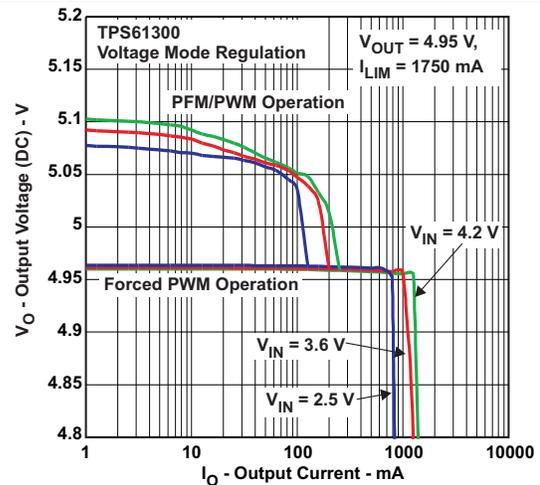
Figure 17. DC Output Voltage vs Load Current
