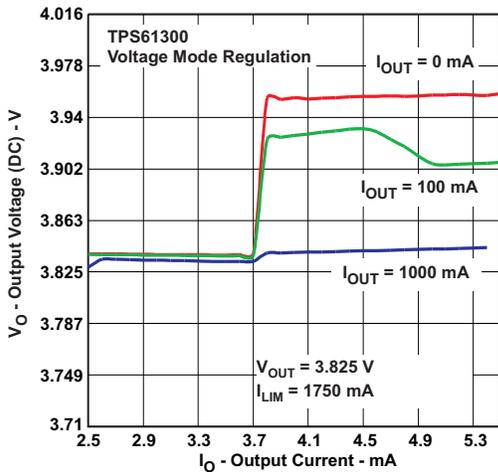
Figure 18. DC Output Voltage vs Load Current
