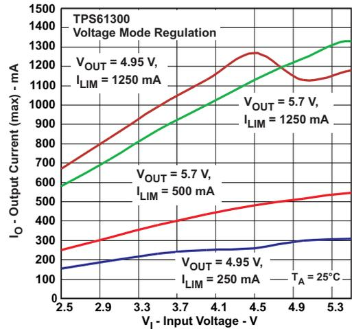
Figure 19. Maximum Output Current vs Input Voltage
