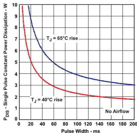
Figure 109. Single Pulse Power Capability
