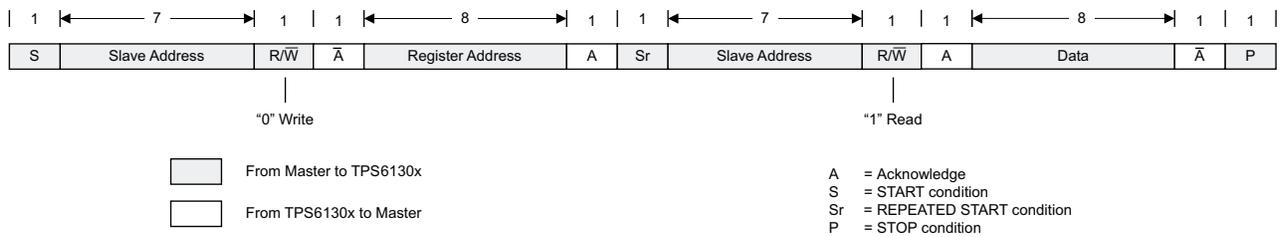
Figure 59. Read Data Transfer Format in F/S-Mode
