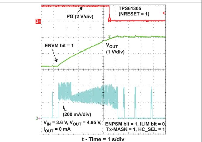
Figure 78. Storage Capacitor Charge-Up (HC\_SEL = 1)
