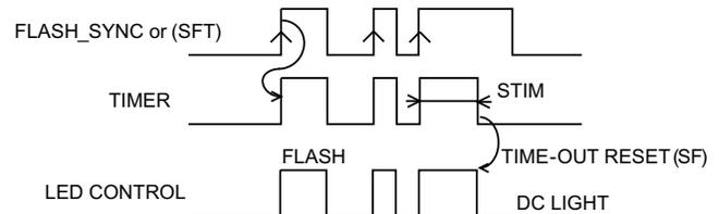
Figure 49. Level Sensitive Safety Timer (Normal Operation + Timeout)
