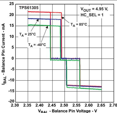
Figure 24. Balancing Current vs Balance Pin Voltage
