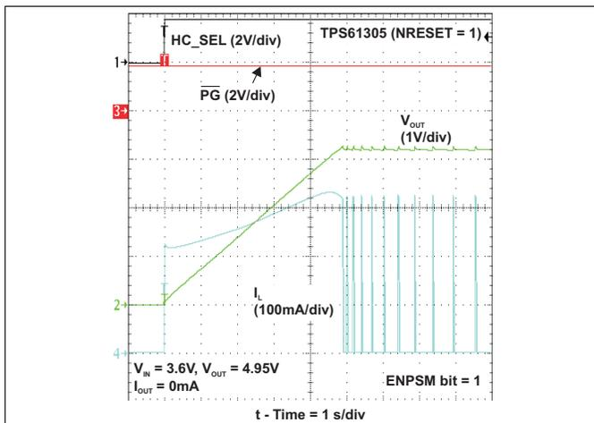
Figure 75. Storage Capacitor Precharge (HC\_SEL = 1)
