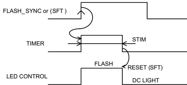
**Figure 50. Edge Sensitive Timer (Single Trigger Event)**
