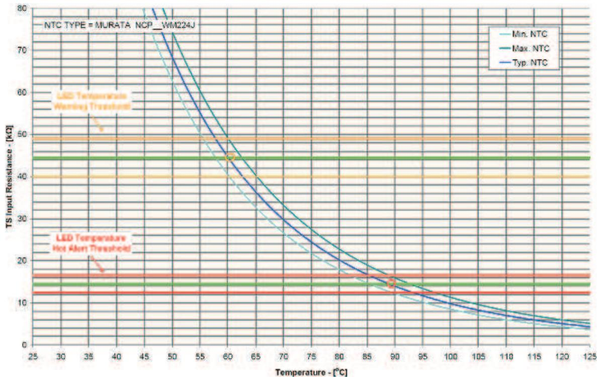
Figure 74. Temperature Monitoring Characteristic
