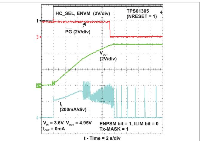
Figure 76. Storage Capacitor Charge-Up (HC\_SEL = 1)
