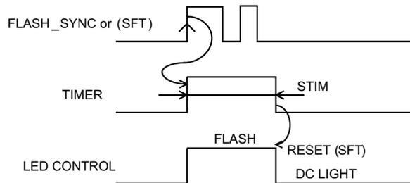
**Figure 52. Edge Sensitive Timer (Multiple Trigger Events)**
