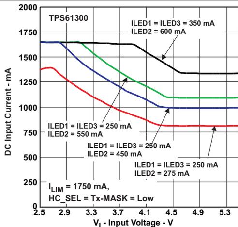
Figure 6. DC Input Current vs Input Voltage
