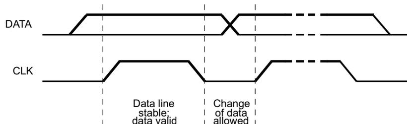
Figure 55. Bit Transfer On the Serial Interface
