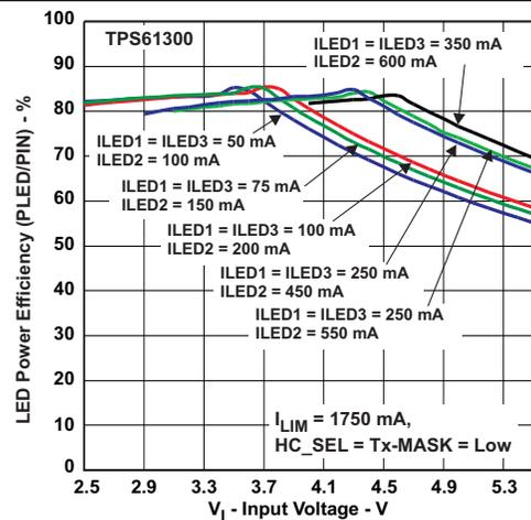
Figure 5. LED Power Efficiency vs Input Voltage
