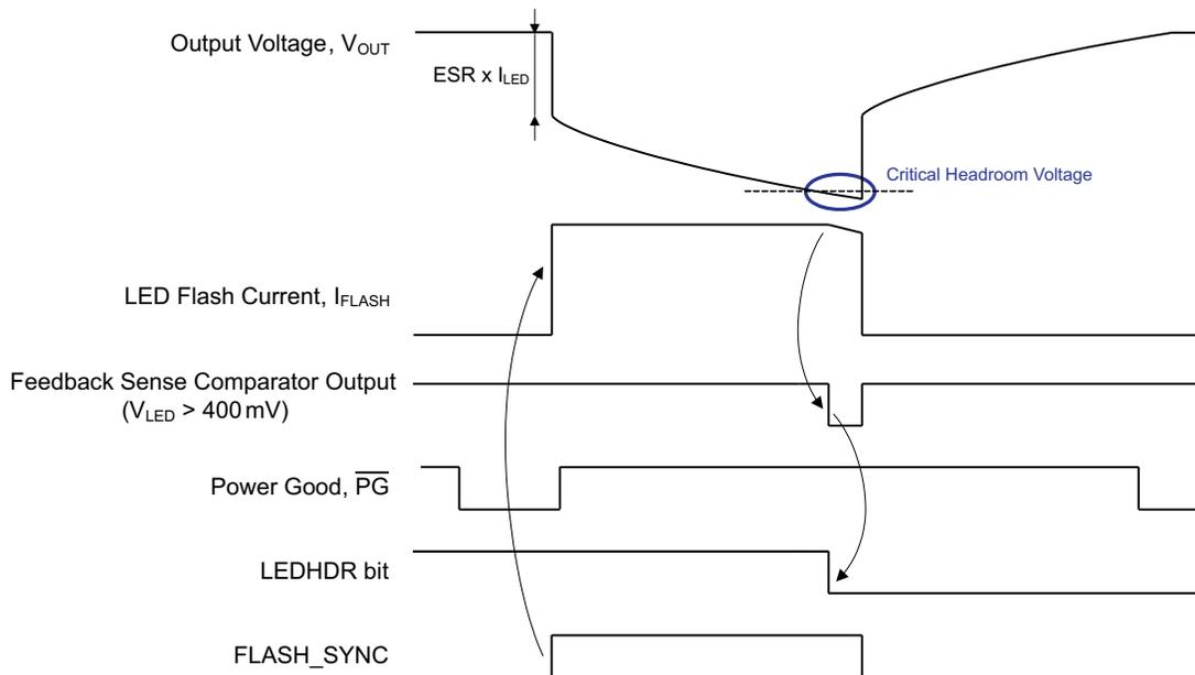
**Figure 43. Storage Capacitor, Simple Adaptive Precharge Voltage**
