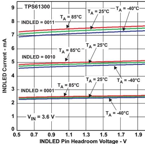
Figure 14. INDLED Current vs INDLED Pin Headroom Voltage
