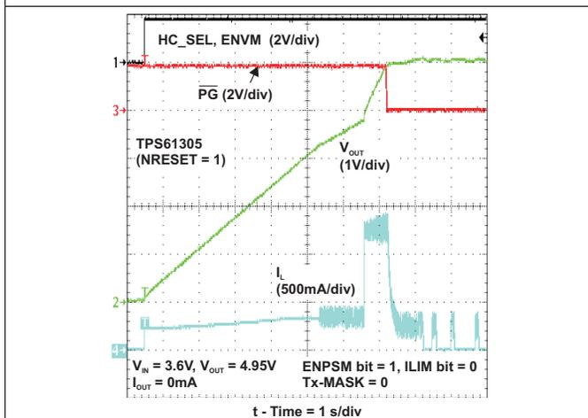
Figure 77. Storage Capacitor Charge-Up (HC\_SEL = 1)
