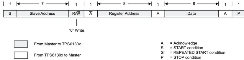
Figure 58. Write Data Transfer Format in F/S-Mode
