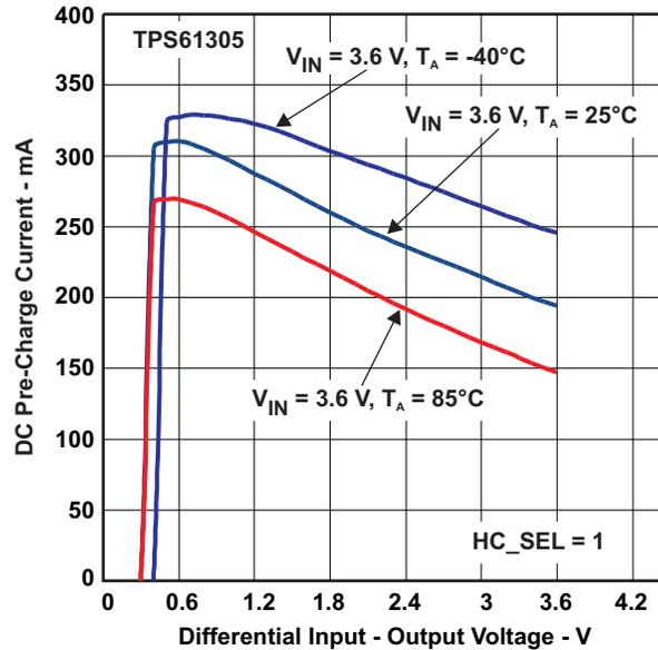
Figure 36. Typical DC Precharge and Short-Circuit Current
