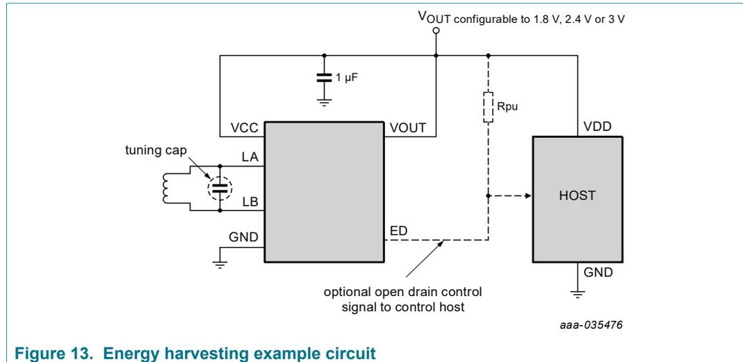
Figure 13. Energy harvesting example circuit
