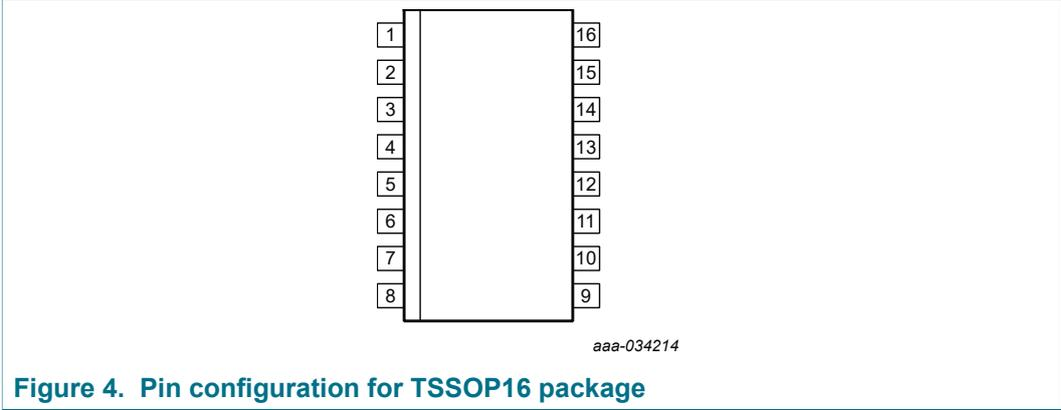
Figure 4. Pin configuration for TSSOP16 package
