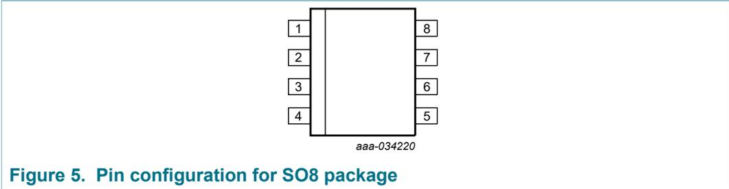
Figure 5. Pin configuration for SO8 package
