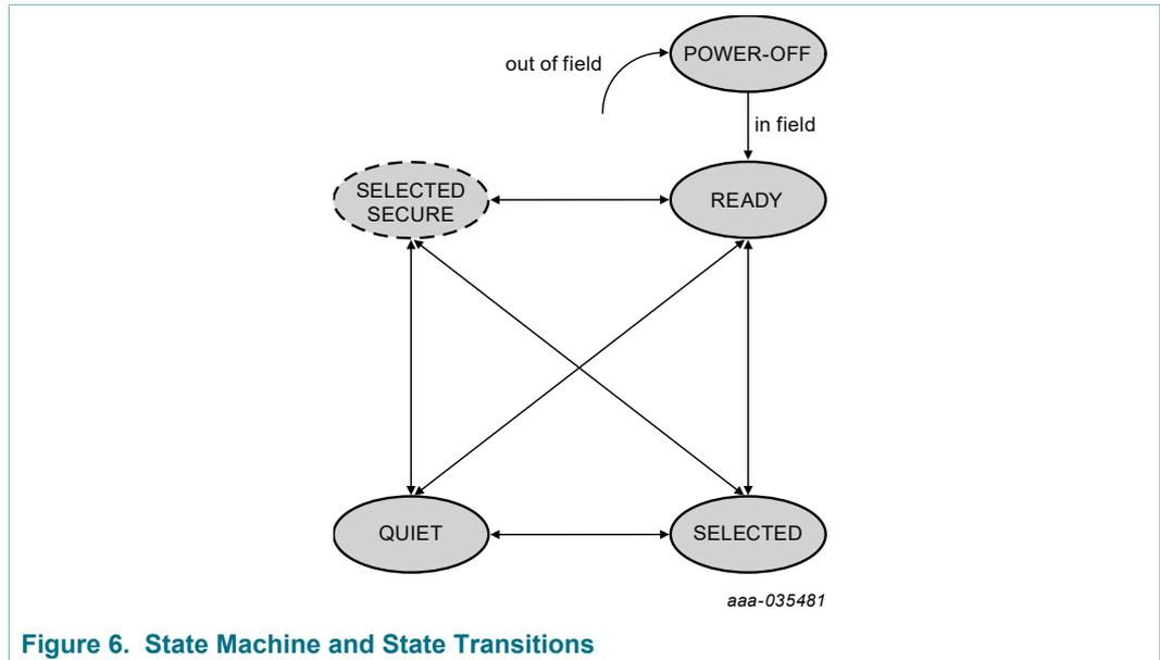
Figure 6. State Machine and State Transitions
