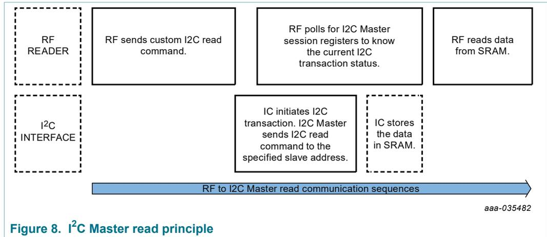
Figure 8. I<sup>2</sup>C Master read principle
