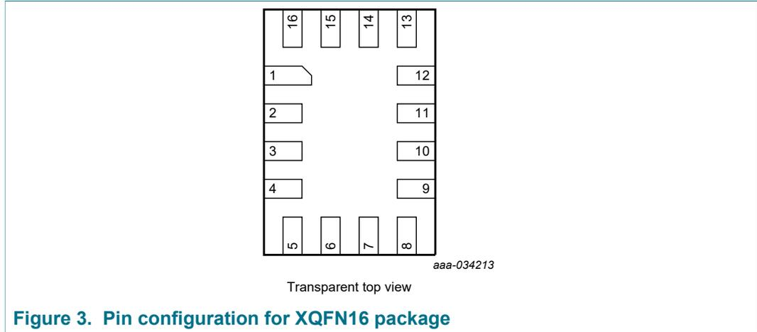
Figure 3. Pin configuration for XQFN16 package
