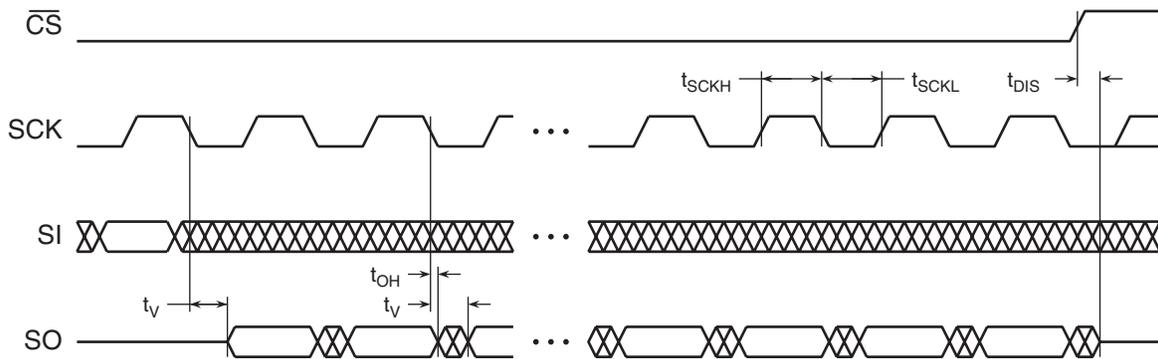
Figure 13-3.  $\overline{WP}$  Timing for Write Status Register Command When SPRL = 1
