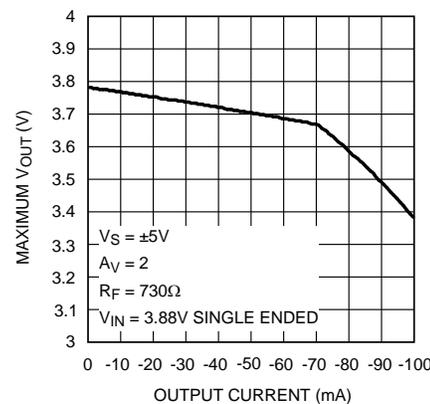
Figure 12. Maximum V<sub>OUT</sub> vs I<sub>OUT</sub>
