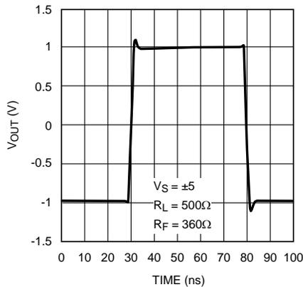
Figure 7. 2 V<sub>PP</sub> Pulse Response Single-Ended Input
