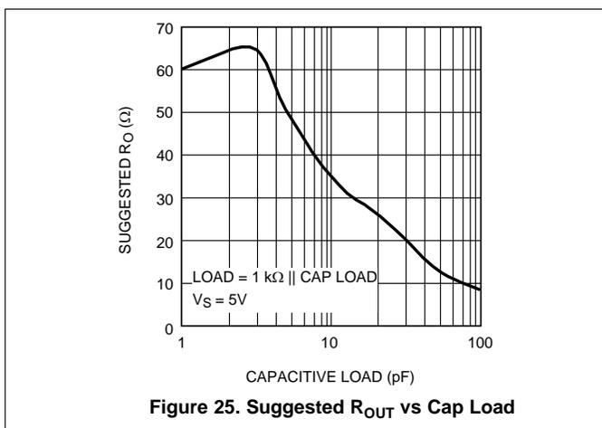
Figure 25. Suggested R<sub>OUT</sub> vs Cap Load
