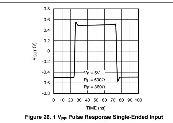
Figure 26. 1 V<sub>PP</sub> Pulse Response Single-Ended Input
