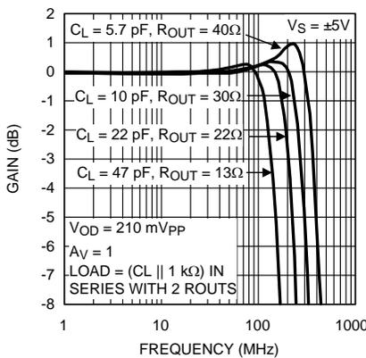
Figure 5. Frequency Response vs Capacitive Load
