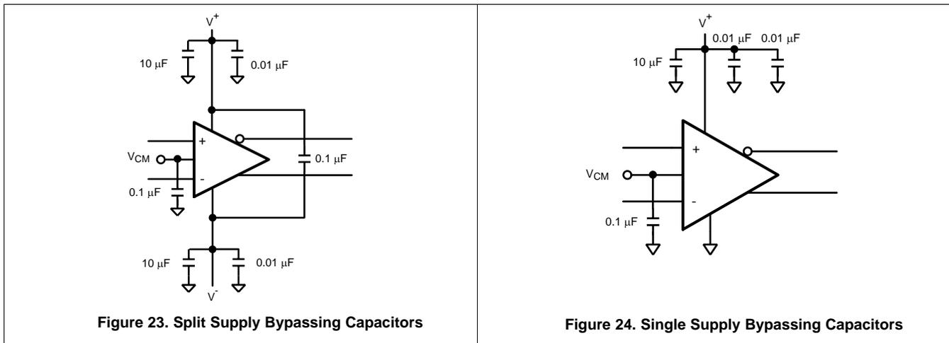
Figure 23. Split Supply Bypassing Capacitors
