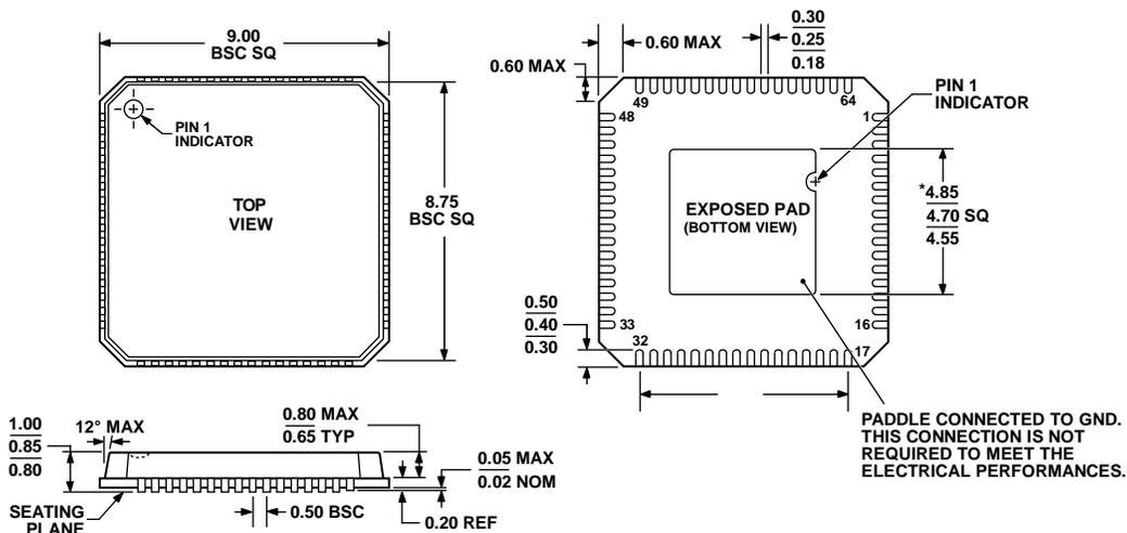
\*COMPLIANT TO JEDEC STANDARDS MO-220-VMM4-4 EXCEPT FOR EXPOSED PAD DIMENSION
