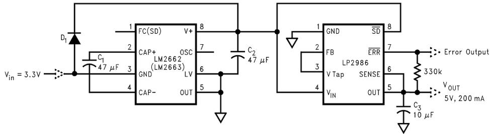
Figure 23. Generating +5 V From +3.3 V Input Voltage
