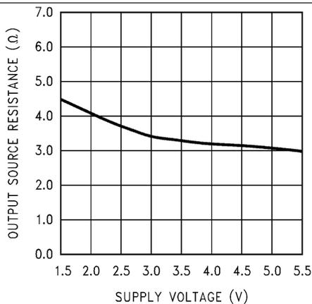
Figure 3. Output Source Resistance vs Supply Voltage
