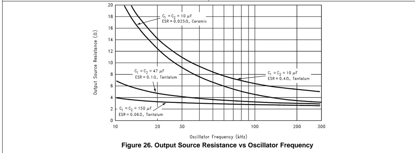
Figure 26. Output Source Resistance vs Oscillator Frequency
