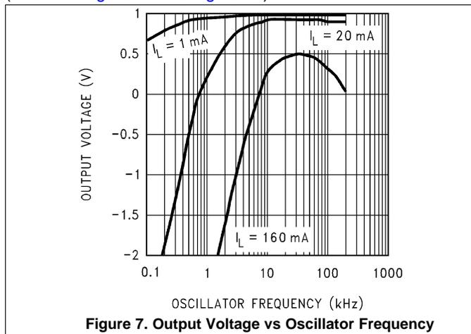
Figure 7. Output Voltage vs Oscillator Frequency
