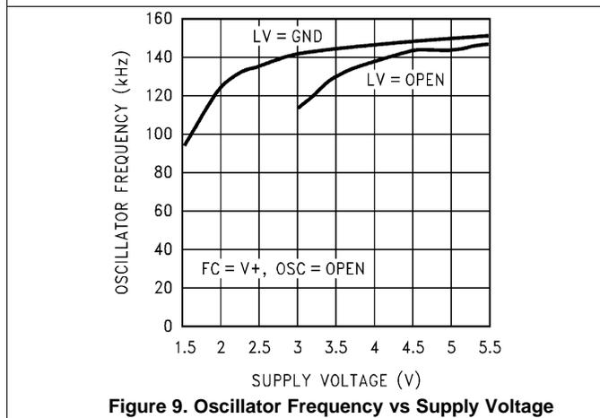
Figure 9. Oscillator Frequency vs Supply Voltage
