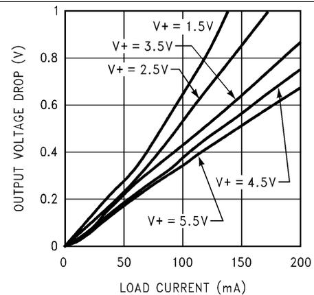
Figure 6. Output Voltage Drop vs Load Current
