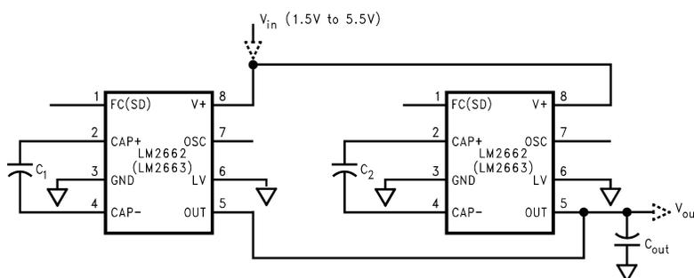
Figure 18. Lowering Output Resistance by Paralleling Devices
