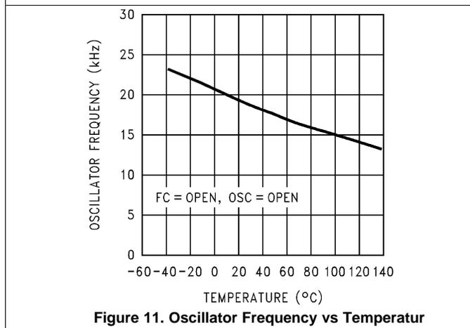
Figure 11. Oscillator Frequency vs Temperature
