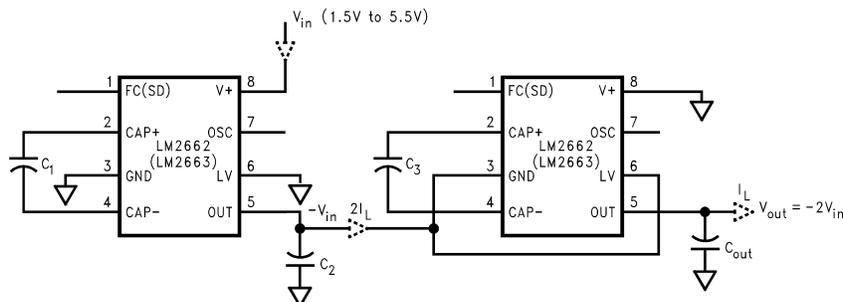
Figure 19. Increasing Output Voltage by Cascading Devices
