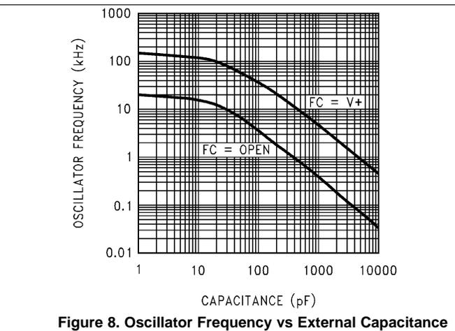
Figure 8. Oscillator Frequency vs External Capacitance
