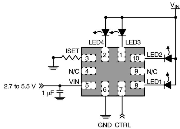
Figure 2. FAN5624 Typical Application for 4 LEDs
