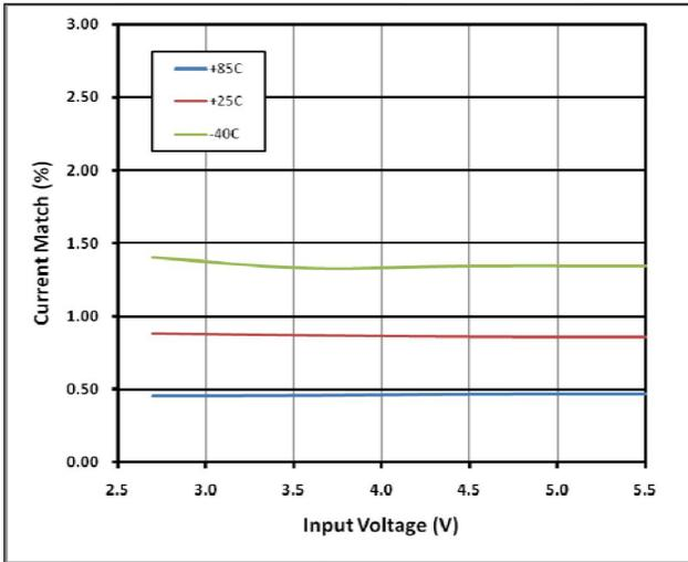
Figure 10. Current Match of Channels vs. Input Voltage
