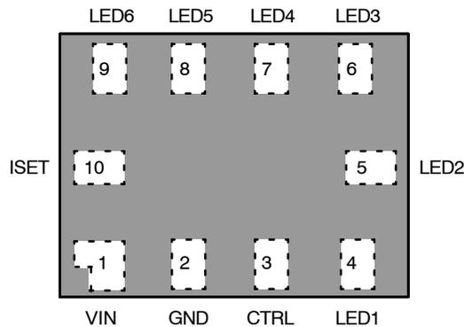
Figure 7. FAN5626: 10-Lead MicroPak MLP, Top View
