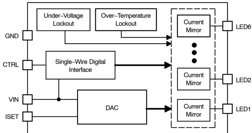
Figure 4. Block Diagram
