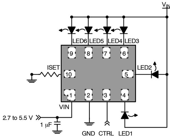
Figure 3. FAN5626 Typical Application for 6 LEDs
