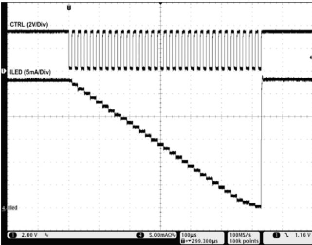
Figure 16. Dimming Operation
