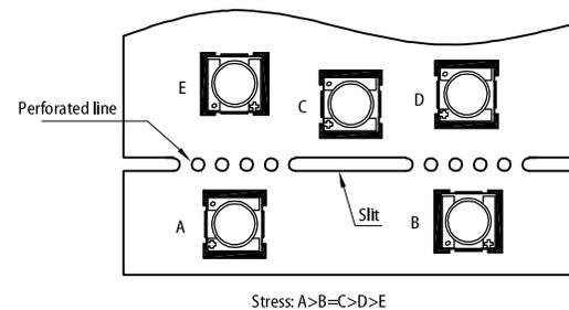
Appropriate LED mounting is to place perpendicularly against the stress affected side.
