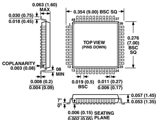
CONTROLLING DIMENSIONS ARE IN MILLIMETERS; INCH DIMENSIONS ARE ROUNDED-OFF MILLIMETER EQUIVALENTS FOR REFERENCE ONLY AND ARE NOT APPROPRIATE FOR USE IN DESIGN
