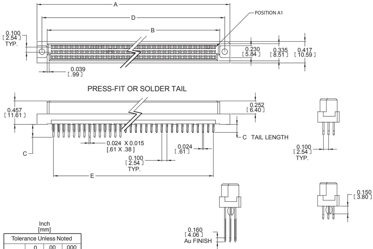
Feed/Thru Wire Strap W, PW1 and PW2 with RR and GG30 Finish (Au both ends)
