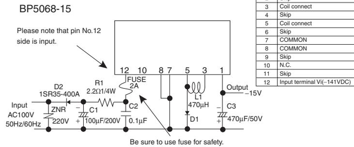
For actual usage, Please kindly evaluate and confirm our part mounted in your product, Especially, Please make sure to confirm the load current does not exceed Max. rated current by using the current probe.
